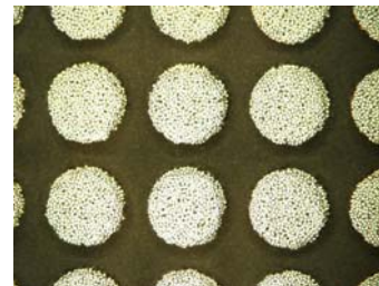
Figure 2: Paste screening for solder fillet
