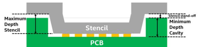
**Figure 9.** Illustration of PCB and stencil tolerance impacting stencil stand-off
