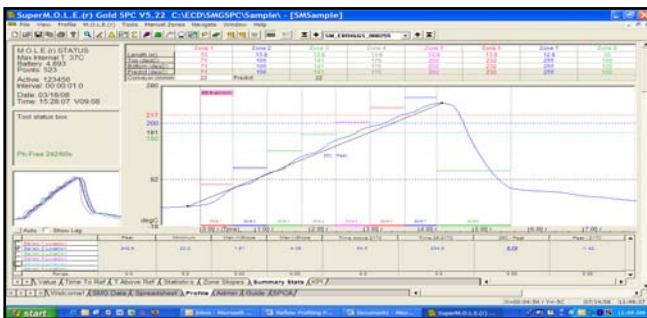
Figure 3 - Note that the maximum slope (1.61°C/second) does not equate to the average ramp rate (0.78°C/second).
