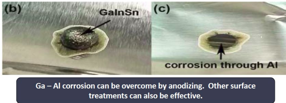
Figure 18. [9] Gallium will dissolve (corrode) aluminum. Anodizing the aluminum may alleviate this concern.
