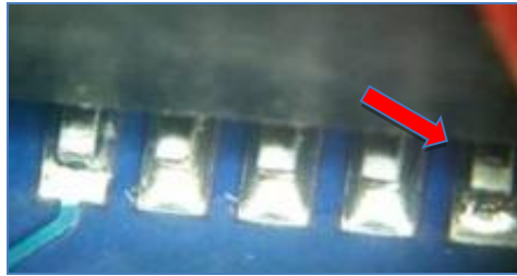
Figure 1. Open Solder on SMT Connector
