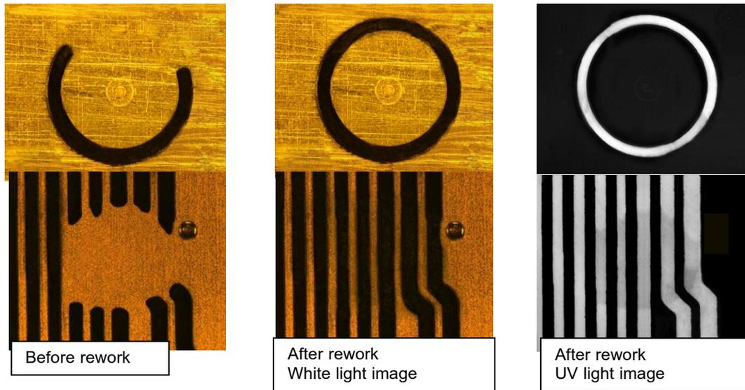
**Figure 3 - Examples Before and After AOR**
