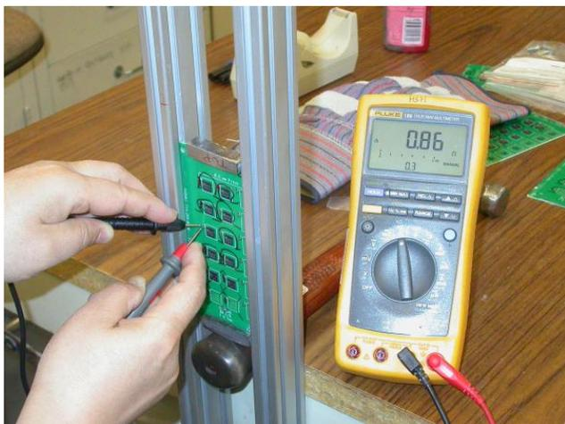
**Figure 16** Component resistance measurement at every 50 drops.
