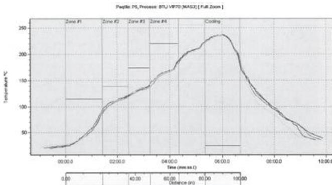
**Figure 8** Reflow profile used in this study
