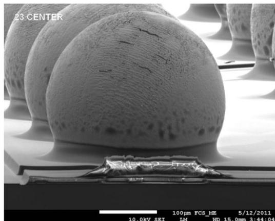
**Figure 21** WLCSP ball mounting with epoxy flux E.
