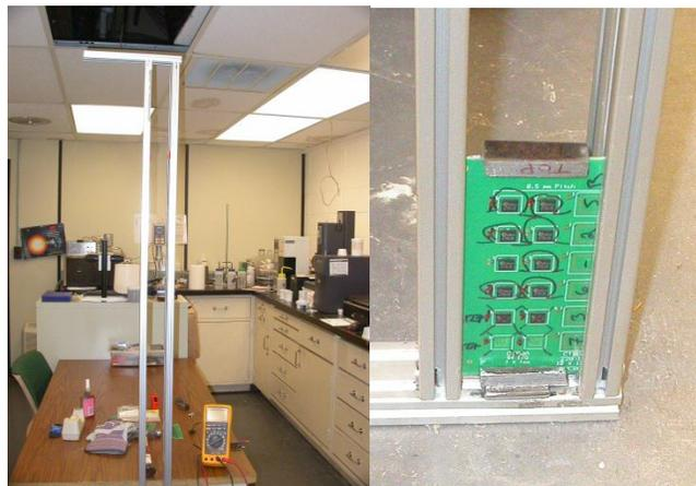
**Figure 15** Frame for drop test setup (left), with a test board already landed on the bottom of test frame (right).
