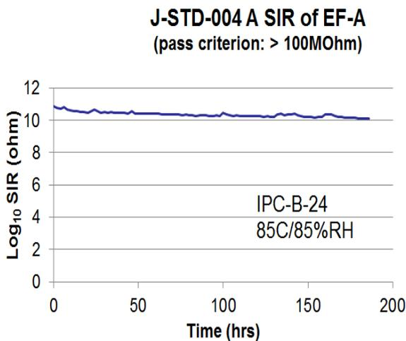
**Figure 18** SIR of epoxy flux A per J-STD-004A
