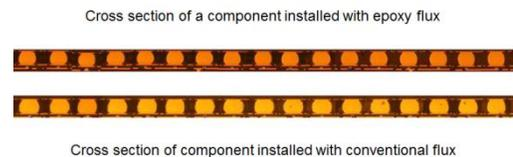
**Figure 9** Cross-section of the BGA assembled, with Epoxy Flux A on the top and conventional flux at the bottom.
