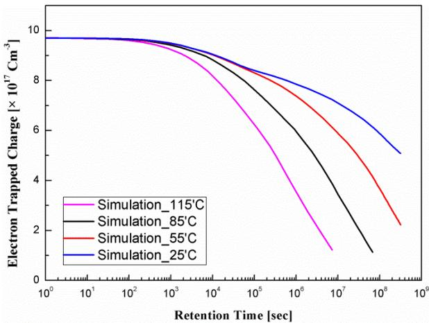
**Figure 11.** Results of electron trapped charges varying with different temperature over time
