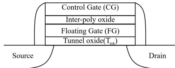
**Figure 1.** Schematic cell configuration of NAND flash memory [4]
