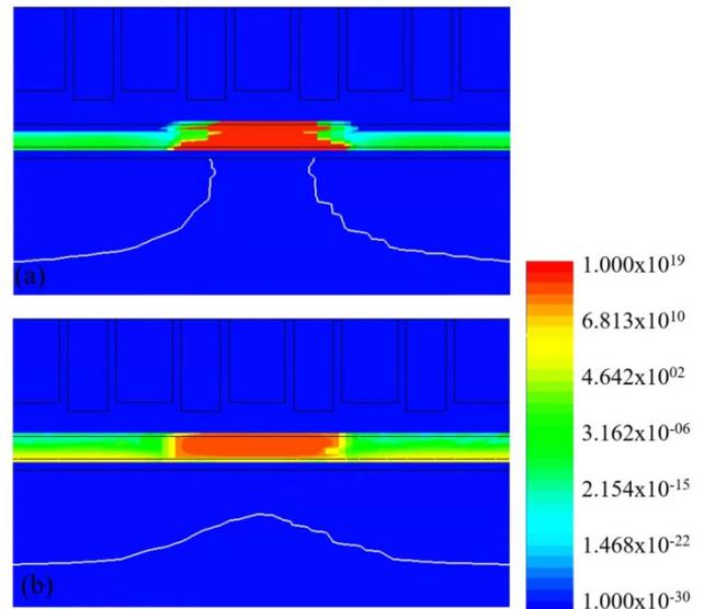
**Figure 9.** Variation of trapped charges by data retention simulation at 85 °C: (a) initial, and (b) 10 year later
