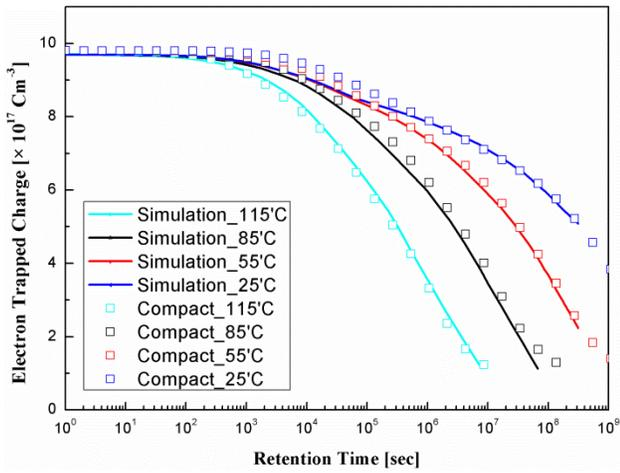
**Figure 13.** Comparison of simulation results and compact modeling results
