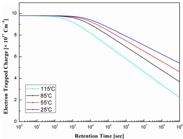
**Figure 15.** Compact modeling behavior of the 4th term by temperature
