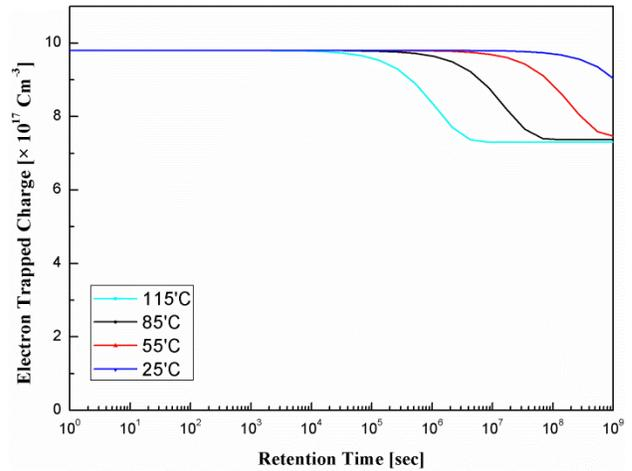
**Figure 14.** Compact modeling behavior of the third term by temperature
