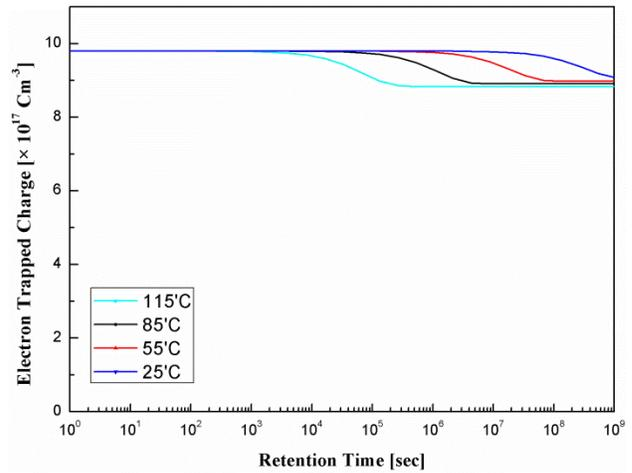
**Figure 14.** Compact modeling behavior of the first term by temperature
