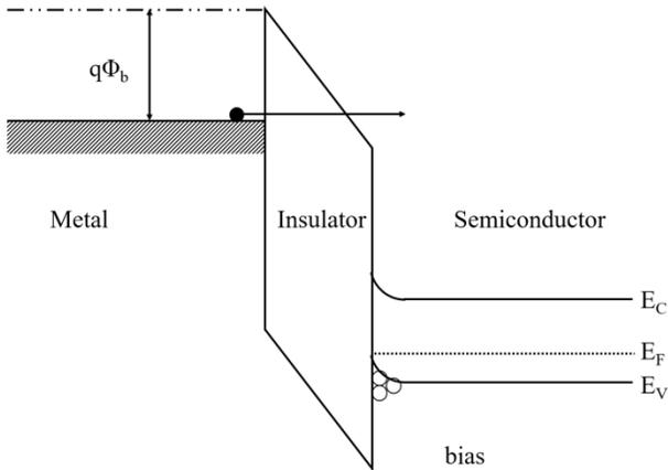
**Figure 2.** Schematic energy band diagram of FN tunneling [5]
