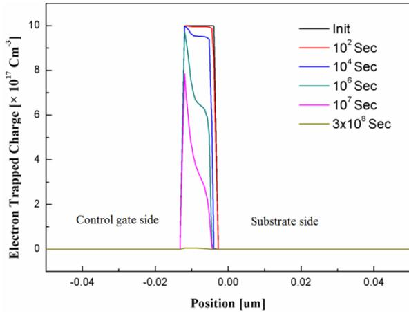
**Figure 10.** Electron trapped charge profile by the location over time (vertical outline direction)
