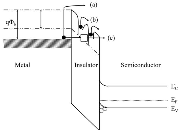
**Figure 4.** Schematic energy band diagram in metal-insulator-semiconductor conduction: (a) Schottky emission, (b) Poole-Frenkel emission, and (c) Trap-assisted tunneling [5, 6]
