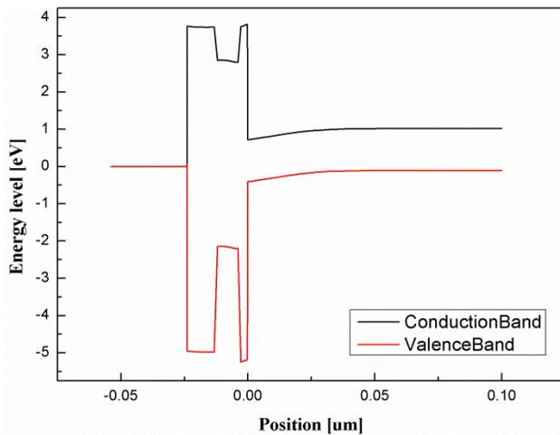
**Figure 7.** Energy band diagram of the simulated TANOS structure (vertical direction)
