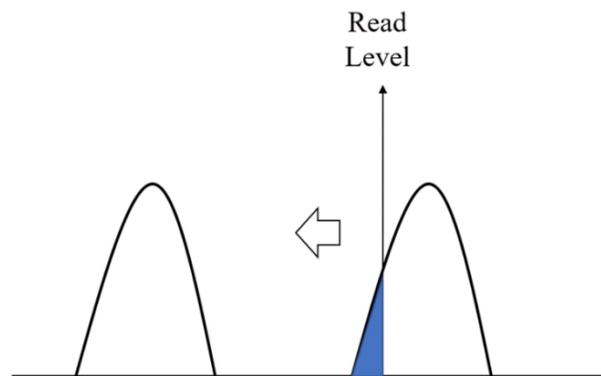
**Figure 5.** Schematic of  $V_{th}$  distribution and counting fail bits [4]
