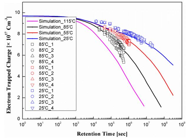
**Figure 12.** Comparison of experimental and simulated data by temperature over time
