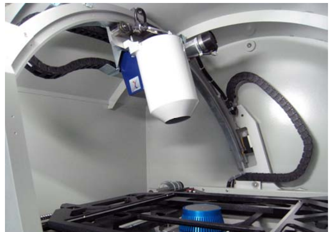
Figure 4. X-ray inspection system with image intensifier (II) detector seen above a sealed-transmissive x-ray tube (sample not present). The detector is held in a cradle mechanism that allows oblique angle x-ray views to be achieved without losing the available magnification on the sample.
