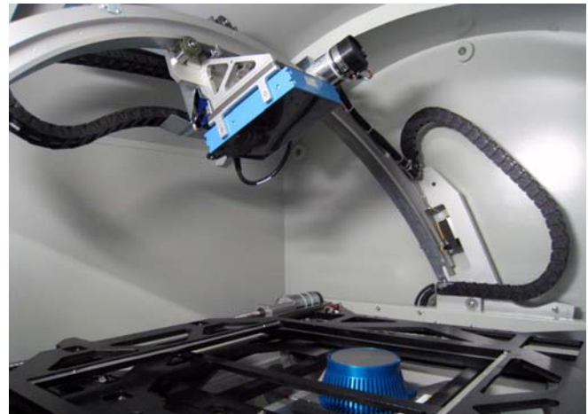
Figure 5. X-ray inspection system with wafer-based-silicon flat panel detector (w-FPD) seen above a sealed-transmissive x-ray tube (sample not present).
