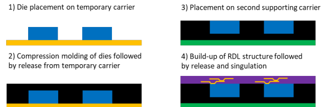
Figure 8: Fan-Out process principal “die first, face-down” [7]
