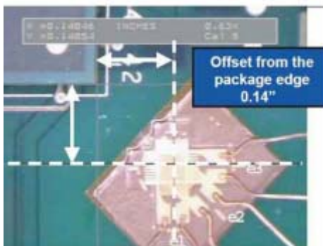
Figure 2: Recommended Gage Placement for BGA Components (IPC-9704)
