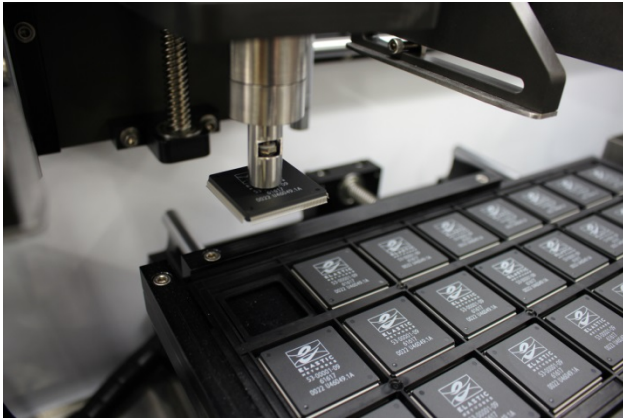
Figure 4. JEDEC tray-to-tray handling system capable of hands-off re-tinning of QFP devices
