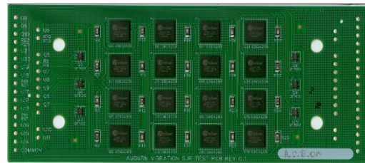
Figure 1: Test board design and manufactured board assembly
