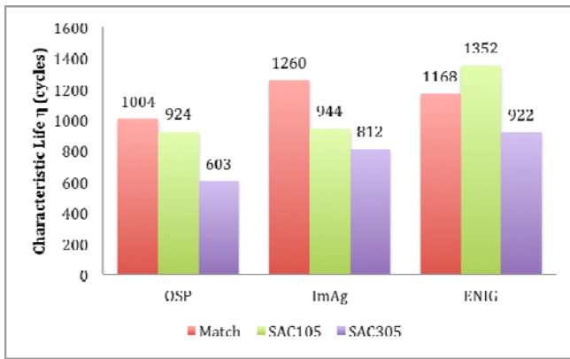
Figure 5. Characteristic Life values for 15mm BGA with Paste A.
