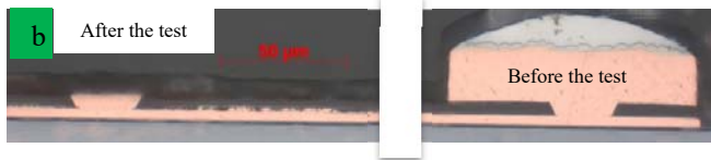
Figure 10. (a) The shear strength of the pillars after reflow, (b) the optical micrographs showing the failure of the pillar after shearing.
