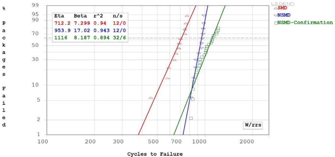
**Figure 22.** Two Parameter Weibull Plot of the -40 to 125°C Thermal Cycling Failures for SMD and NSMD PCB Pads.
