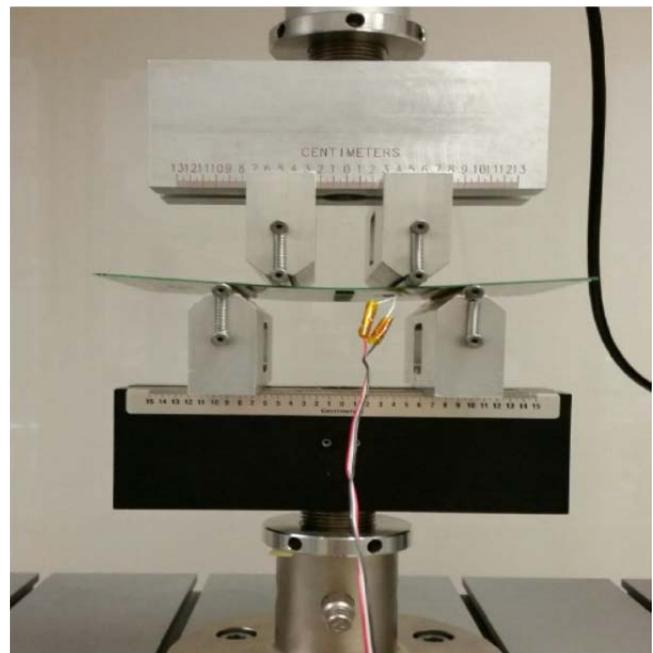
**Figure 23.** Four Point Monotonic Bend Test Configuration.
