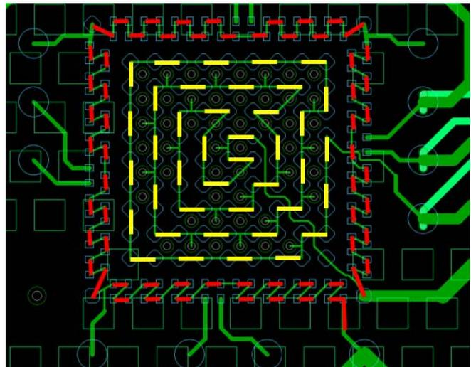
**Figure 11.** Top Down View of 211 FC PLGA Daisy-Chain Routing with the PCB (Green) and Package (Red and Yellow) Nets Both Shown. I/O's Not Included in the LGA Daisy-Chain Were Assigned to Monitor the Bump Connections.
