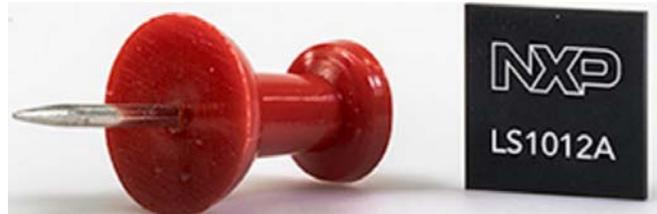
**Figure 1.** 211 FC PLGA Topside Image with Thumbtack Shown for Relative Size Comparison.
