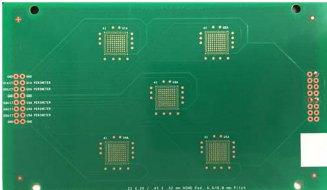
**Figure 13.** Unpopulated JEDEC Drop Test Board.
