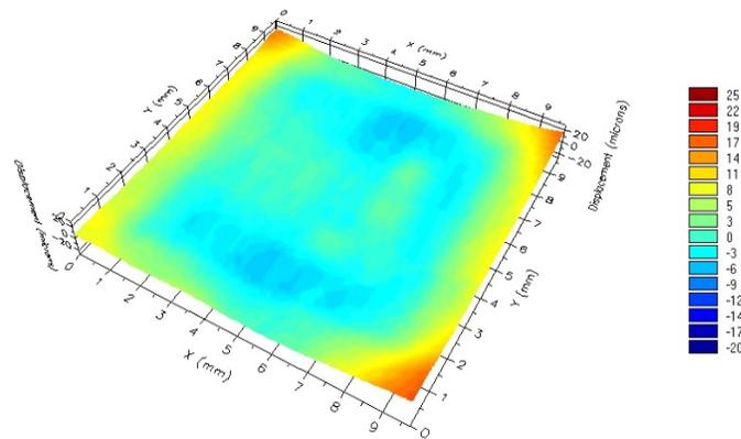
**Figure 9.** Typical 3D TherMoiré Plot of Bottomside FC PLGA Warpage of 23  $\mu\text{m}$  at Peak 260°C Reflow.
