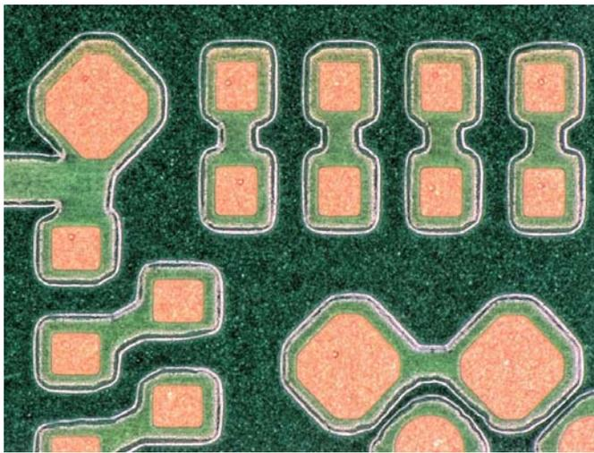
**Figure 15.** A Portion of the Daisy-Chain Footprint that Uses SMD Pads with a 50 µm Soldermask Overlap of the Copper Pads.
