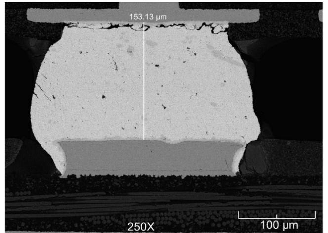
**Figure 21.** Cross-Section of a Typical Failing NSMD PCB Joint. Note Fracturing Predominantly at Package Interface.
