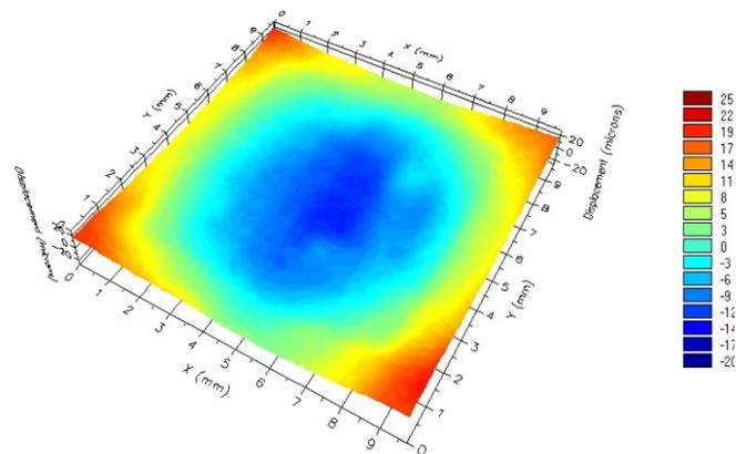
**Figure 8.** Typical 3D TherMoiré Plot of Bottomside FC PLGA Warpage of 34  $\mu\text{m}$  at Room Temperature of 25°C.
