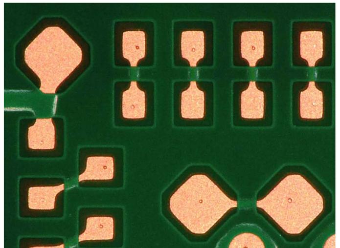
**Figure 14.** A Portion of the Daisy-Chain Footprint that Uses NSMD Pads with a 50 μm Soldermask Clearance Around the Copper Pads. Marks Visible on Pads are from PCB Test.
