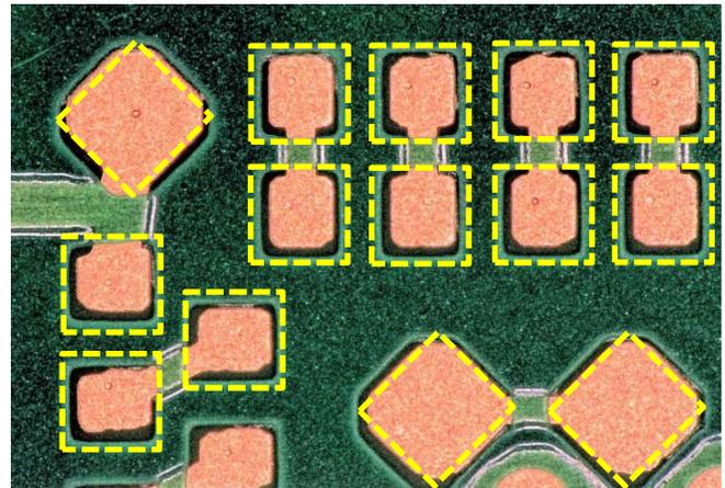
**Figure 17.** The SMD PCB Footprint Shown Overlaid with an Improved Stencil Design in Dashed Yellow Lines Where the Perimeter Pads had Aperture Openings with a 1.61:1 Ratio to the Pads. This Allowed for a Theoretical 60% Overprint on Those Pads.
