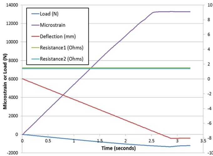
**Figure 24.** Plot of Microstrain, Load, Deflection and Electrical Resistance Versus Time During Bend Testing. The Load, and Therefore Deflection and Microstrain, Maxed Out Around 13,000  $\mu$ strain with No Failures Recorded.
