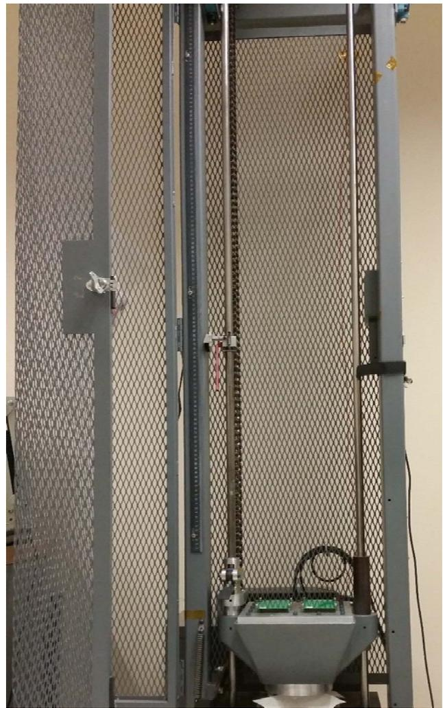
**Figure 25.** Shock Tower with Two Attached PCBs Used for Electrically Monitored JEDEC Drop Testing to 1500 Gs.
