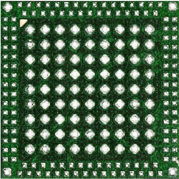
**Figure 2.** 211 FC PLGA Bottomside Image Showing Two Outer Rows of LGA Pads at 0.5 mm Pitch and 0.8 mm Pitch Inner 9 × 9 Array of LGA Pads.
