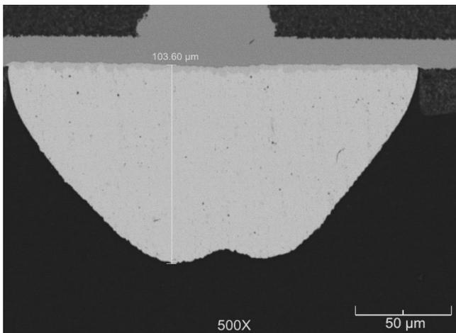
**Figure 7.** 500X SEM Image of a Cross-Section of an Approximately 100  $\mu\text{m}$  SnAgCu Solder Bump on an Outer LGA Pad. Note the Bump Height Measurement of 103.60  $\mu\text{m}$  and the Test Mark on the Bump.
