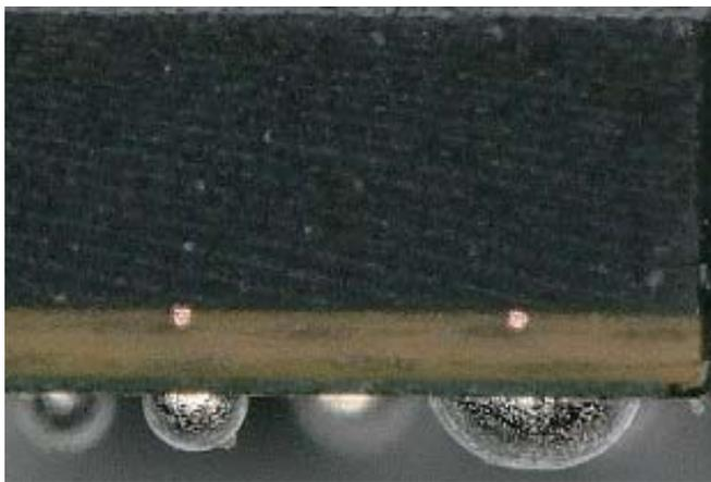
**Figure 6.** Optical Image Showing FC PLGA Substrate, Mold Compound and the 100  $\mu\text{m}$  of Pre-Applied Solder Bumps on the LGA Pads.
