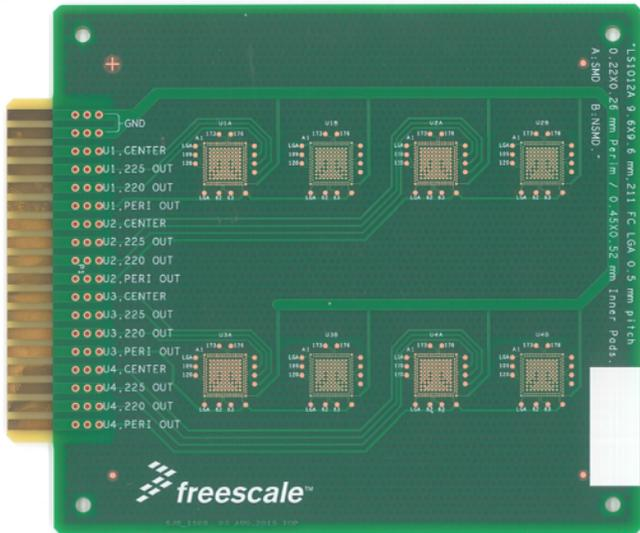
**Figure 12.** Unpopulated Thermal Cycling Test Board. Note the Hard Gold Plated Edge Fingers on the Left Side Are for Continuous, In-Situ Monitoring in the Chamber. This PCB Was Also Used for Bend Testing.
