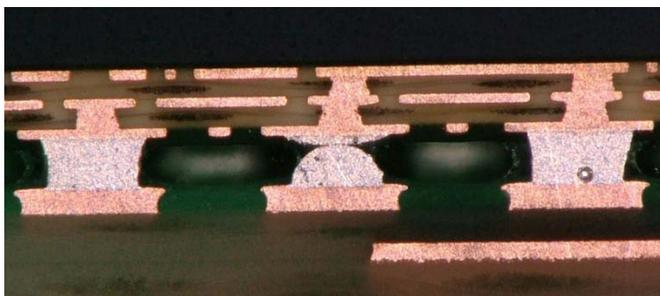
**Figure 16.** Low Solder Paste Volume Induced Open on the Perimeter Row of LGA Joints Encountered When Using
