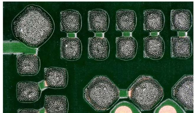
**Figure 18.** Solder Paste from a Typical Stencil Print Using Improved Stencil with Openings with a 1.61:1 Ratio on the 0.5 mm Pitch Perimeter Pads Only.
