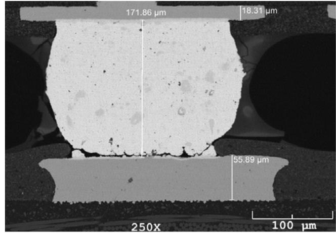
**Figure 20.** Cross-Section of a Typical Failing SMD PCB Joint. Note Fracturing Predominantly Near PCB Pad.
