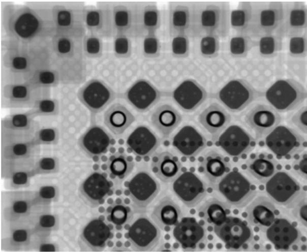
**Figure 19.** Typical X-ray Image Following SMT Assembly Showing Consistent LGA Solder Joints from the 1.61:1 Area Ratio Stencil Apertures. Note the Typical Solder Joint Voiding and the Flip Chip Die Bumps.
