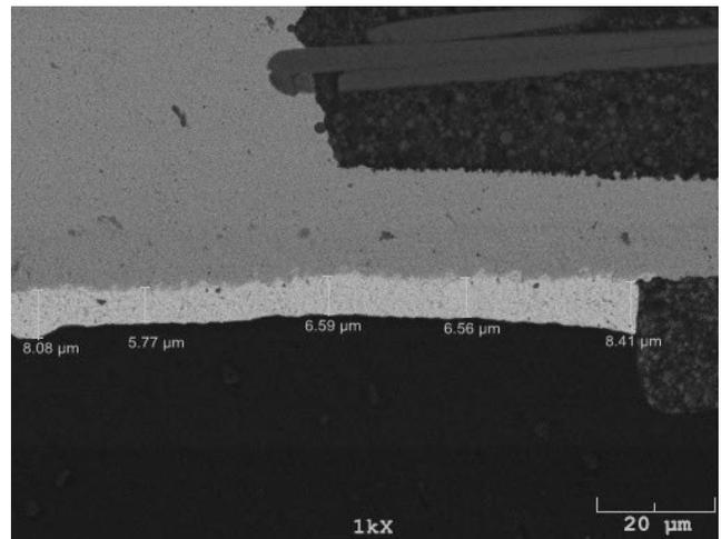
**Figure 5.** 1kX SEM Image of a Cross-Section of a Portion of LGA Pad with Before Additional Solder Was Applied to Pad.
