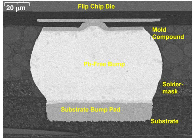
**Figure 4.** Higher Mag (800X) SEM Image of a Typical Pb-Free Bump on the FC PLGA.
