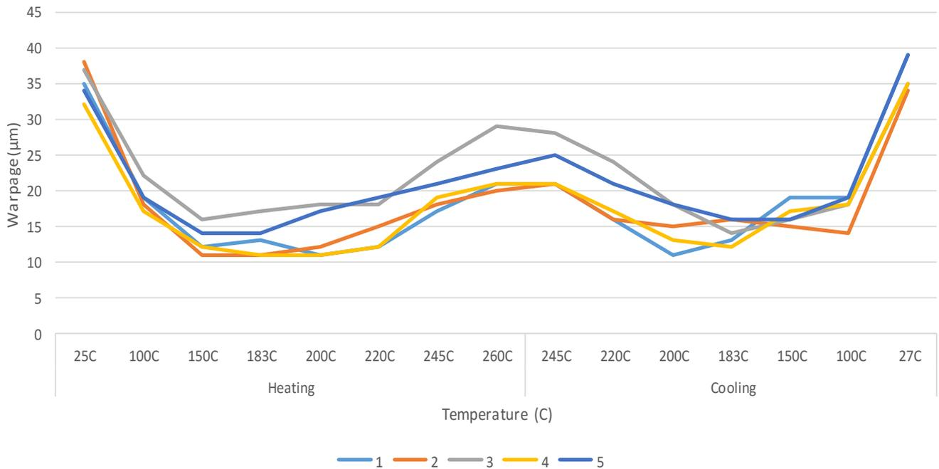
**Figure 10.** TherMoiré Warpage Plot on Five 211 FC PLGAs at 15 Temperatures During a 260°C Peak Reflow Profile.
