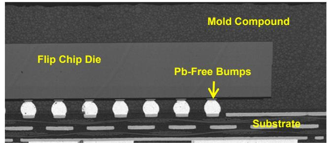
**Figure 3.** Cross-Section of FC PLGA Showing Mold Compound on Both Top and Bottom of the Die, Pb-Free Die Bumps and Three Copper Layer Laminate Substrate.
