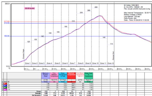
Figure 5. Reflow profile of 2.4mm thick board.
