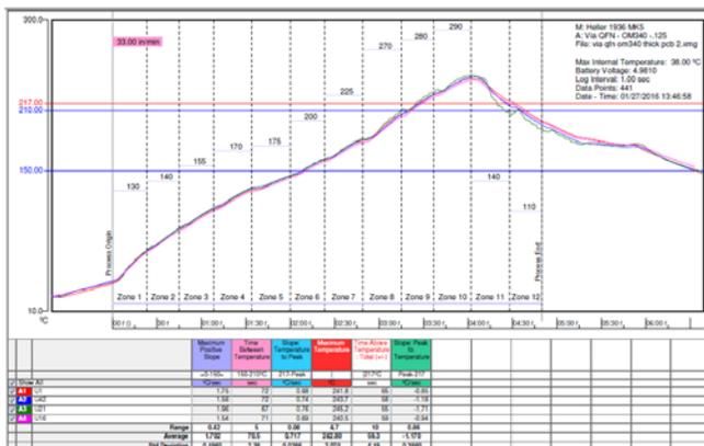
Figure 6. Reflow profile of 3.2mm thick board.
