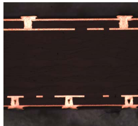
Figure 2: Misplaced air sparger; solution movement only on one side (filled vias)
