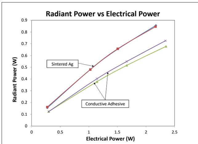
**Figure 5b.** UV LED: Radiant Power vs Electrical Input Power for Sintered Ag vs Conductive Adhesive
