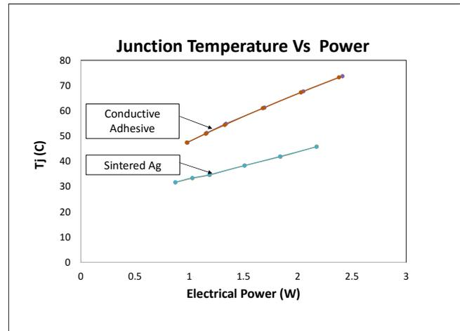
**Figure 5a.** UV LED: Junction Temperature vs Power for Sintered Ag vs Conductive Adhesive
