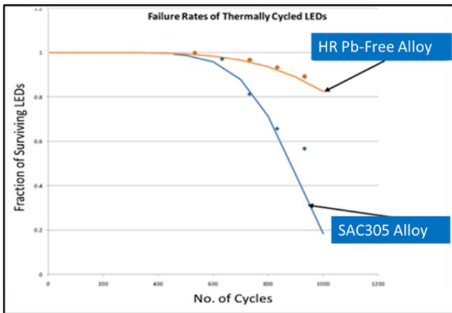
**Figure 3.** Failure rate vs. number of thermal cycles of ceramic submount high power LEDs on MCPCB.
