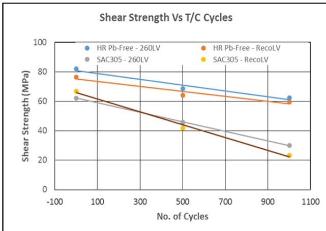
**Figure 4.** Thermal Cycles vs Shear Strength for HR Pb-Free and SAC305 alloys.
