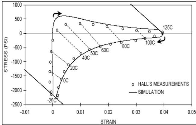
**Figure 2.** Solder Joint Hysteresis Loop During Thermal Cycling Between -25°C and 125°C.
