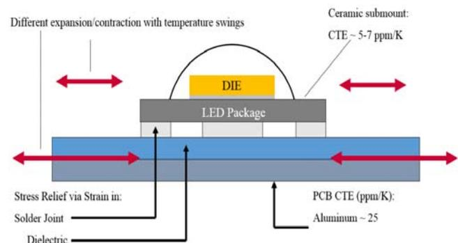
**Figure 1.** Drawing of an Assembled High-Power Ceramic LED on a Metal-Core PCB Showing CTE Differentials.
