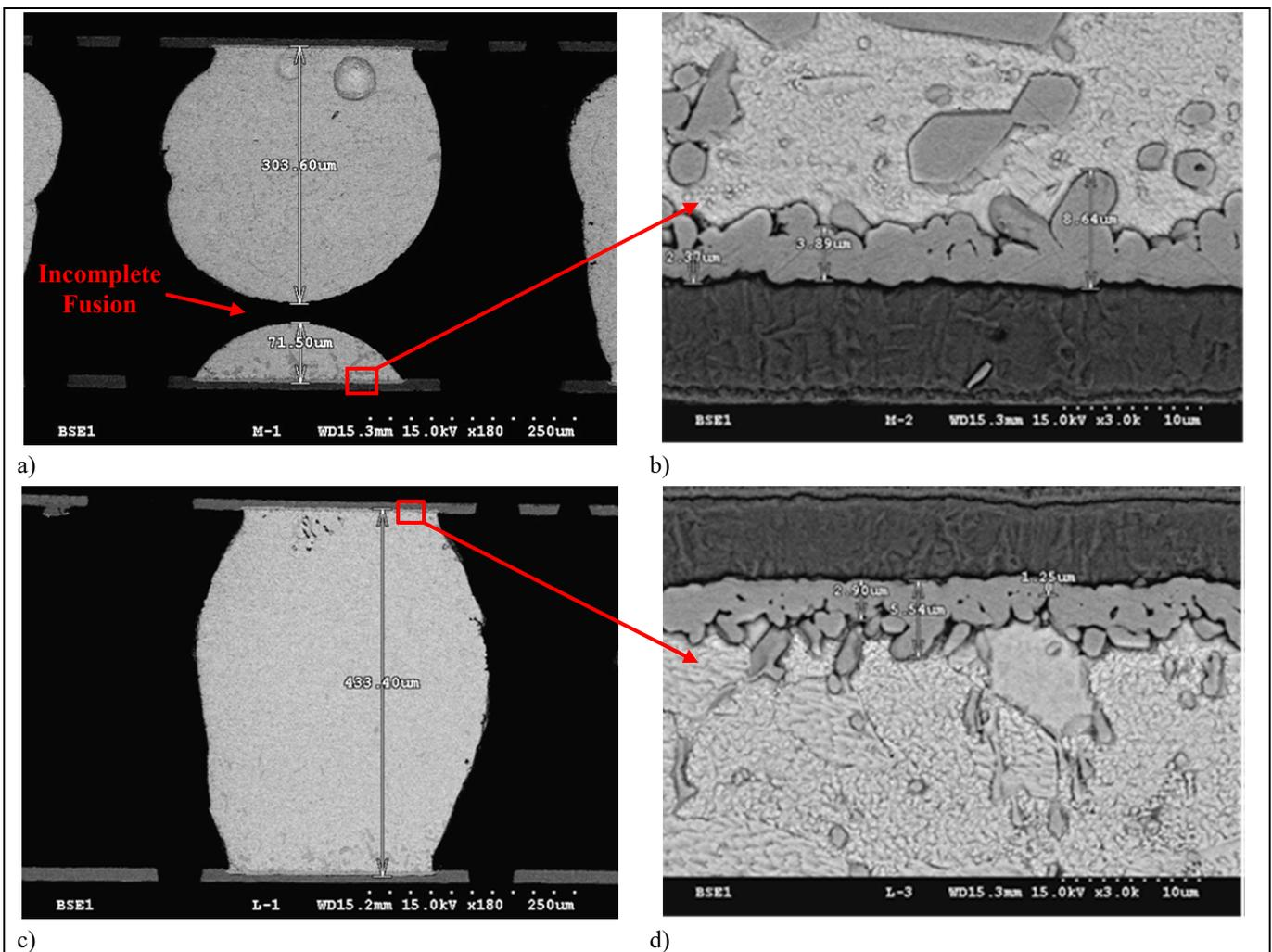
**Figure 4.** Micromorphology of Some Representative Solder Joints in the Top Layer
