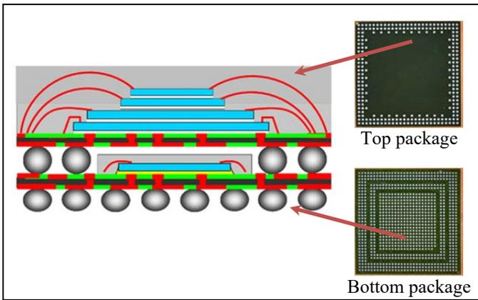
**Figure 10.** PoP Module Model Structure
