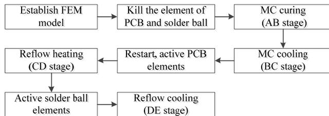
**Figure 13.** Simulation Steps Corresponding to Figure 12
