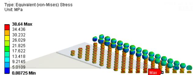
Figure 18. Stress Contour for Solder Joints after Reflow
