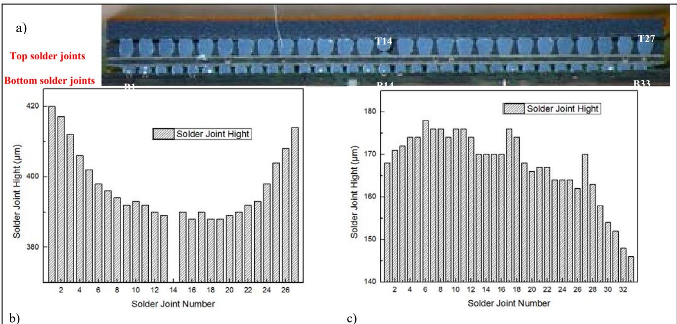
**Figure 3.** Representative Cross-sectional View of PoP Solder Joints and the Measured Height Data
