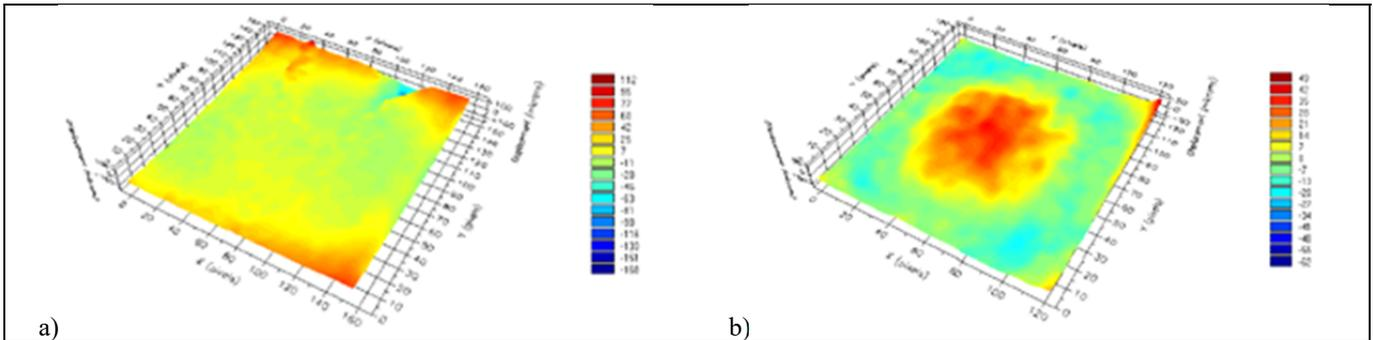
**Figure 9.** Representative 3D Thermo-moiré Plots at the Temperature of 260°C
