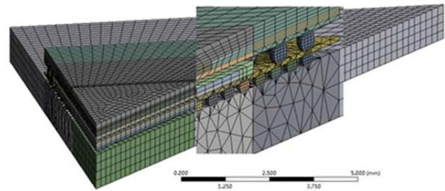
**Figure 11.** Finite Element Model for PoP on Board Level Assembly
