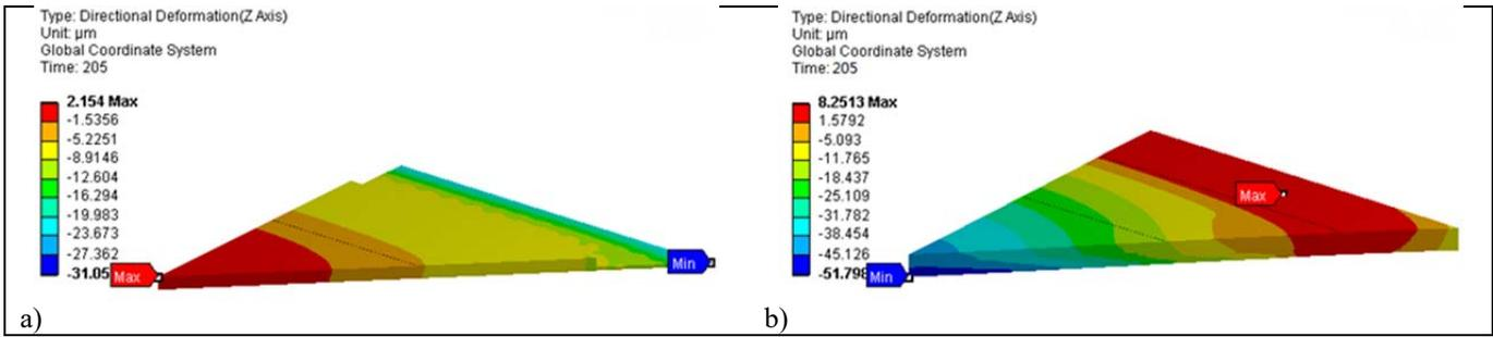
Figure 15 Warpage Patterns after MC Molding for the Packages, a) top package: convex, b) bottom package: concave
