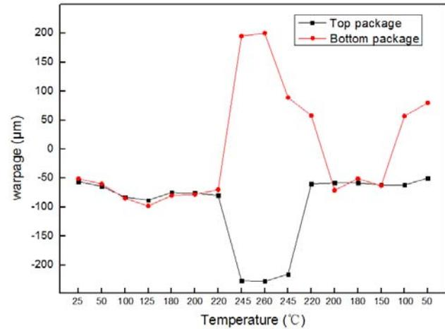
**Figure 8.** Test Results of Warpage Measurement for Top and Bottom Packages
