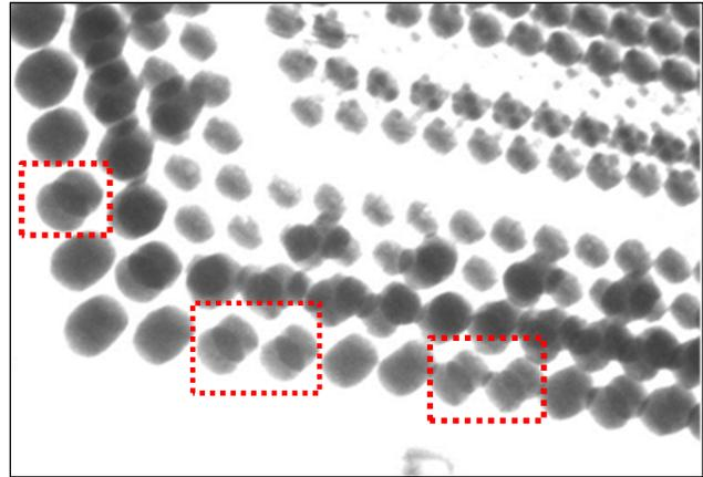
**Figure 2.** Representative Views of X-ray Inspection for the PoP Solder Joints
