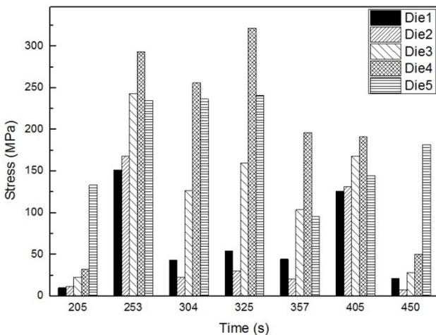
Figure 17. Stress Evolution in Dies during Reflow Process
