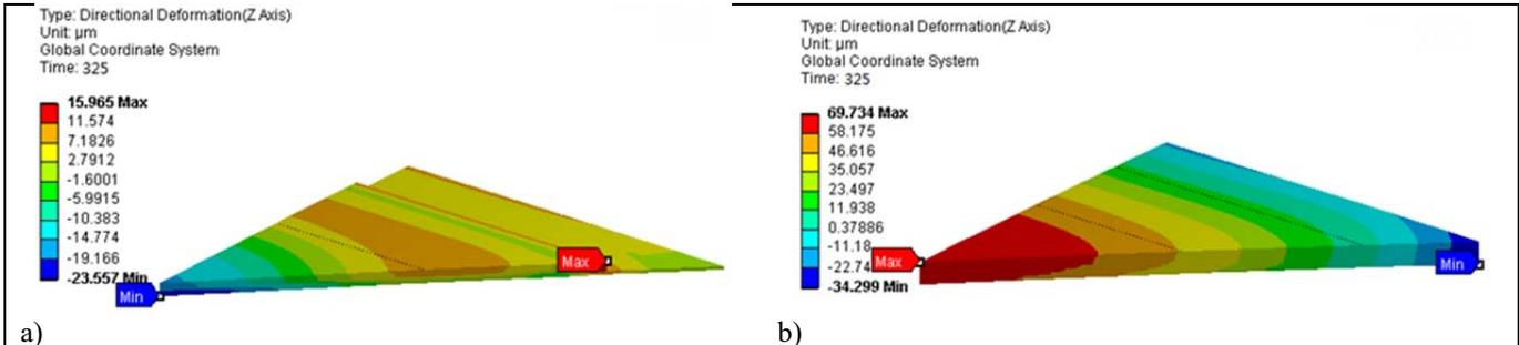
Figure 16. Warpage Patterns at the Reflow Peak Temperature, a) top package: concave; b) bottom package: convex
