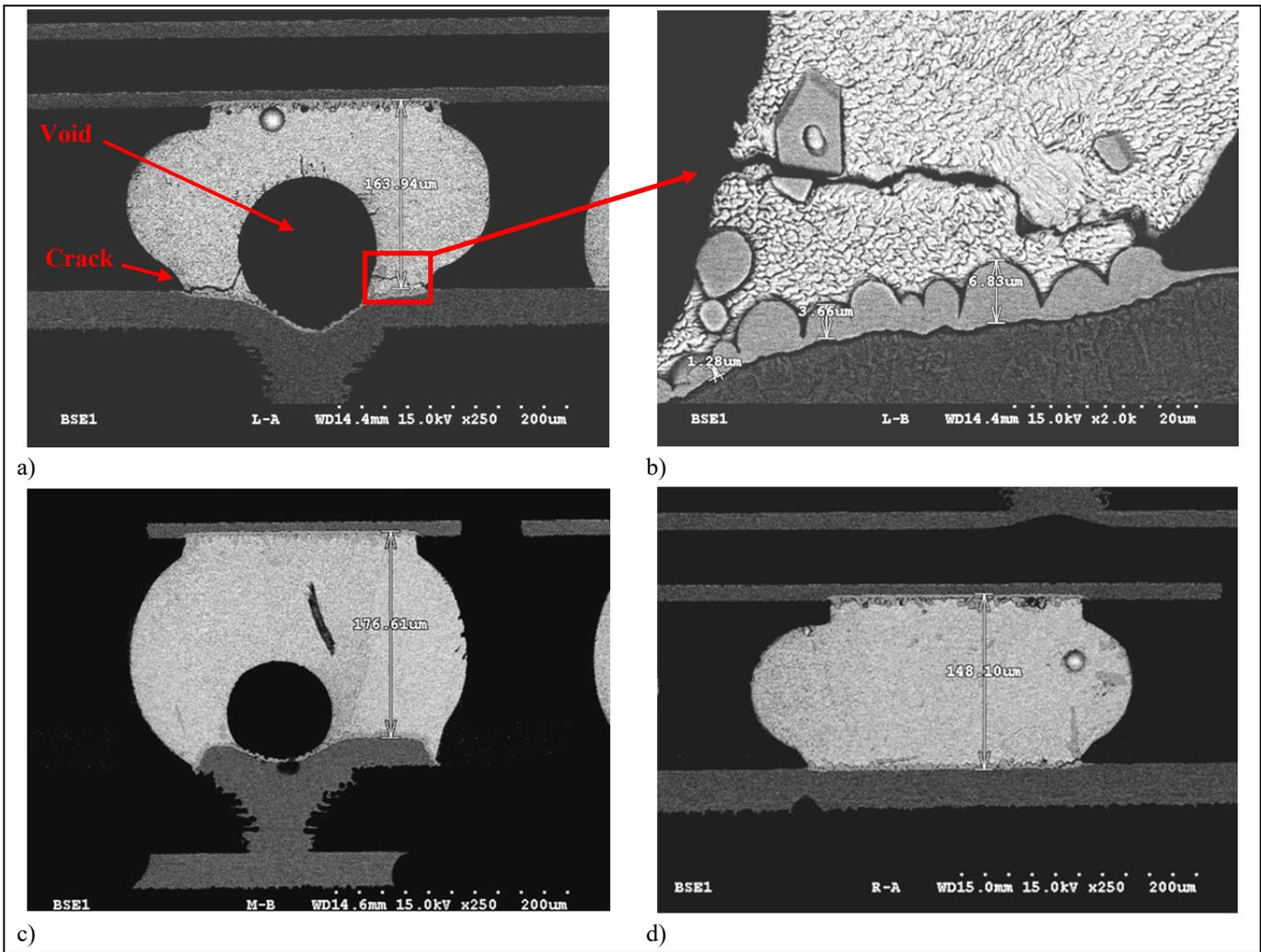
**Figure 5.** Micromorphology of Some Representative Solder Joints in the Bottom Layer
