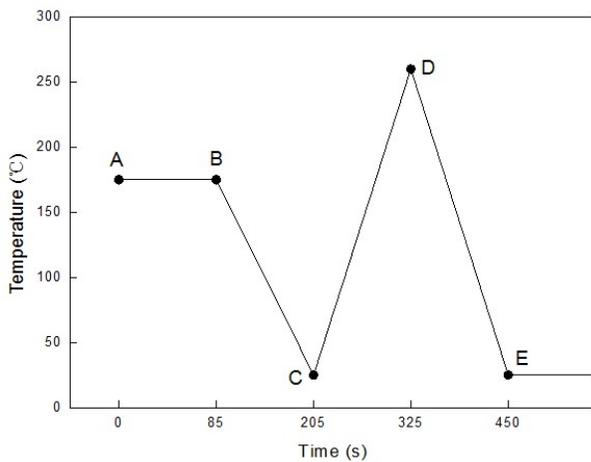
**Figure 12.** Temperature Loading Profile for the Whole Manufacturing Process
