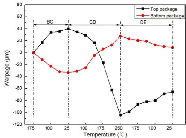
**Figure 14.** Warpage Value Evolution during the Whole Process.
