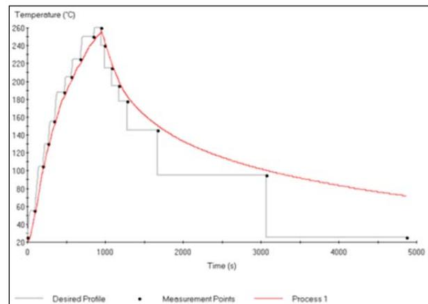
**Figure 6.** Plot of Package Body Temperature vs Time
