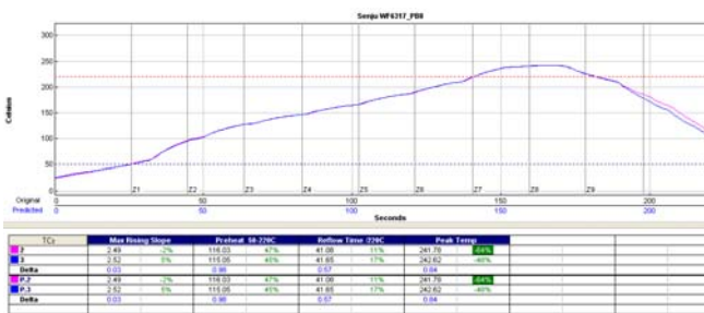
Figure 4. Ramp-To-Peak profile for flux S2
