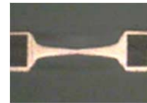
Figure 5. Example of Accelerated Plating at Hole Center
