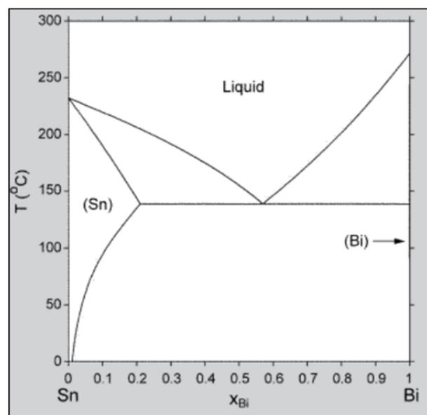
**Figure 4.** (a) Bi-Sn phase diagram [The diagram is from Ref.9]
