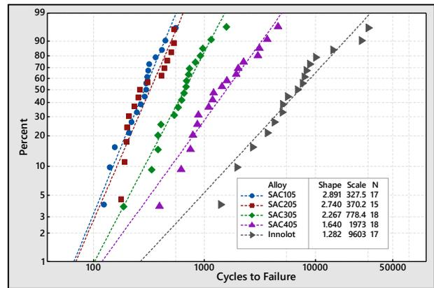
**Figure 3.** Weibull plots showing the effect of composition on the room temperature shear fatigue life of solder joints on Cu-OSP substrates [The data is from Ref. 5].
