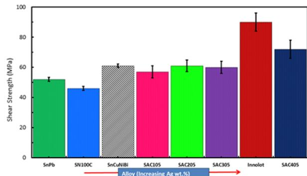
**Figure 11.** Plot of shear strength of 20mil solder joints on Cu-OSP surface finish versus Ag concentration in various solder alloys.
