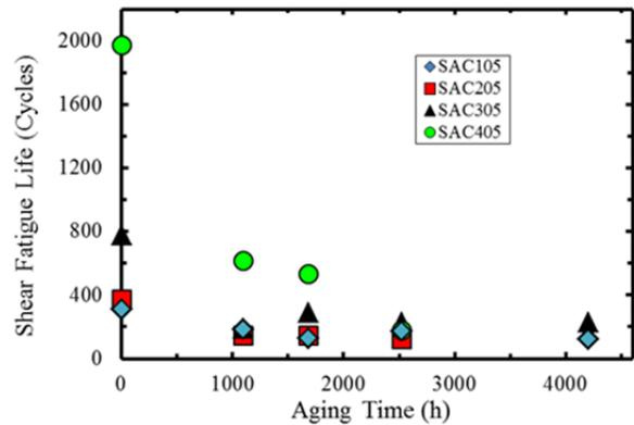
**Figure 13.** The effect of aging on the room temperature shear fatigue characteristic life time of different SAC alloys. The aging temperature was 125°C.
