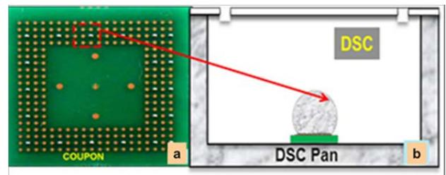
**Figure 6.** Shows (a) Printed Circuit board on which solder joints were built (b) a Printed Circuit Board with a square area delineated by dashed red lines with only one solder bump which is placed in the differential scanning calorimeter (DSC) after dicing.
