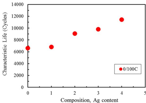
**Figure 2.** A plot of the characteristic lifetime versus Ag concentration in the solder joint, during accelerated thermal cycling of thin chip array ball grid array (CTBGA) SnAgCu solder joints. [The data is from Ref. 4]
