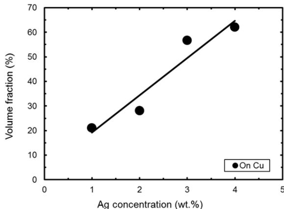
**Figure 10.** A plot of volume fraction of the near eutectic SnAgCu material (interdendritic region filled with  $Ag_3Sn$  and  $Cu_6Sn_5$  precipitates) versus Ag concentration for SnAgCu/Cu solder joints.
