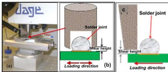
**Figure 7.** (a) Dage4000+ with sample block mounted to a fixture with an arrow pointing to the shear fatigue tool (b) the sketch of the shear fatigue tool (c) The sketch of the set up for the ball shear test.
