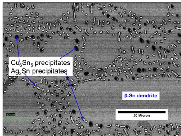
**Figure 1.** A scanning electron micrograph of a near eutectic Sn-Ag-Cu alloy (SAC387). The near eutectic phase can be seen, along with  $\beta\text{-Sn}$  dendrites. Some examples of  $\text{Ag}_3\text{Sn}$  and  $\text{Cu}_6\text{Sn}_5$  precipitates in the near eutectic phase are labeled.
