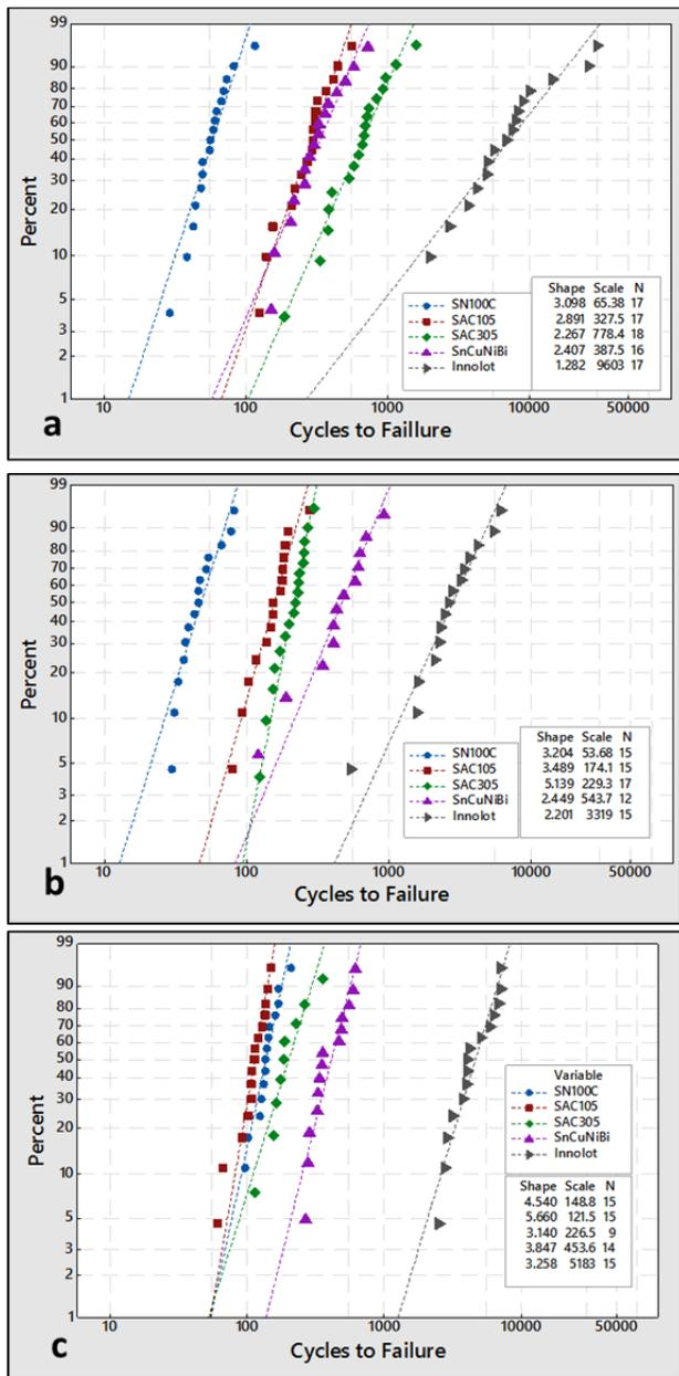
**Figure 12.** Weibull plots showing isothermal shear fatigue performance for sets of 20mil solder joints of five alloys on Cu-OSP substrate, for different aging times (a) as-reflowed, (b) aged at 125°C for 2520 hours (c) aged at 125°C for 4200 hours.
