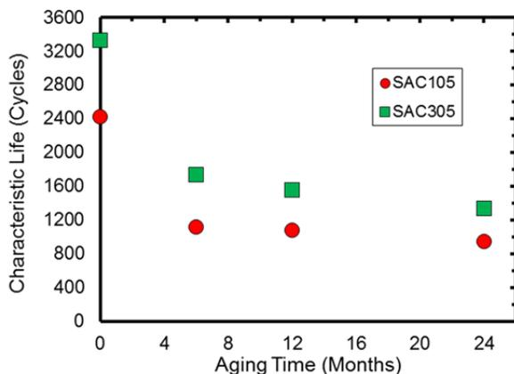
**Figure 5.** A plot of characteristic life versus aging time for 10mm ball grid array (BGA) SAC105 and SAC305 packages aged at a temperature of  $125^\circ\text{C}$  [The data is from Ref. 19].
