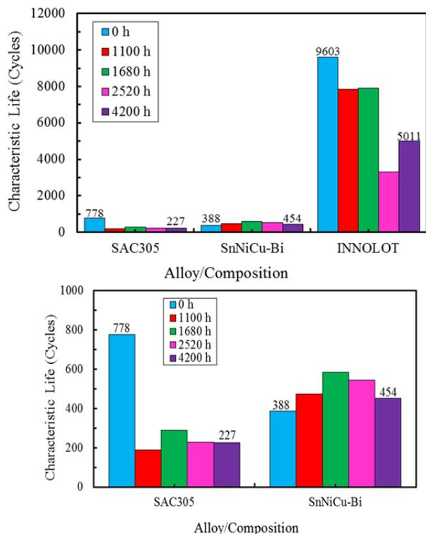
**Figure 14.** Bar charts reveal the effect of aging on the room temperature shear fatigue characteristic life time of different SAC alloys. The aging temperature was 125°C. An expanded version of the bar charts for SAC305 and SnNiCuBi is provided.
