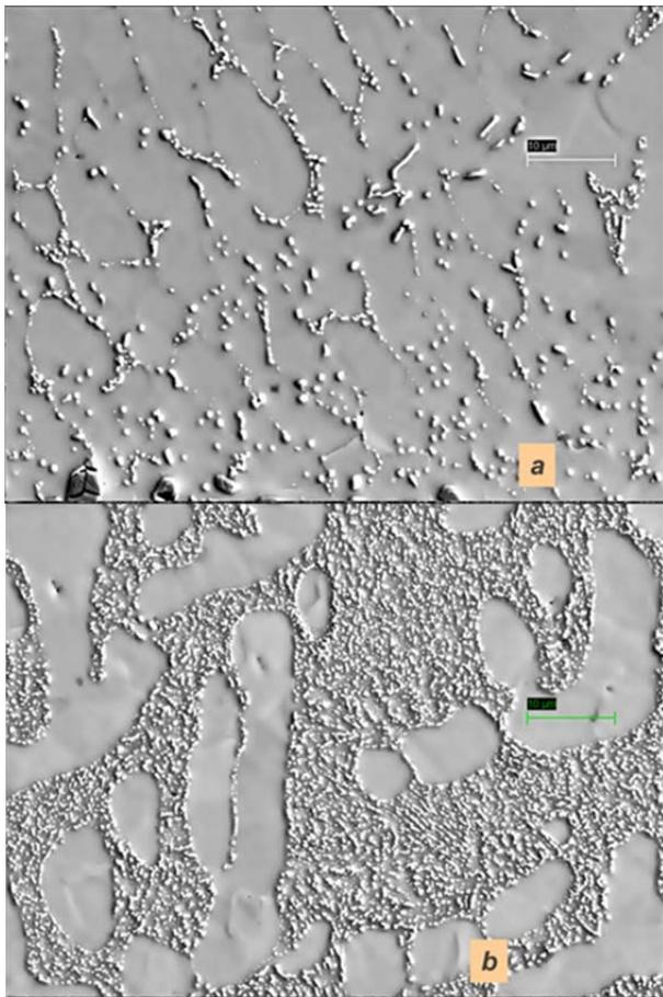
**Figure 9.** Scanning electron microscopy (SEM) images of (a) SAC105 and (b) SAC405 solder joints on Cu substrate.
