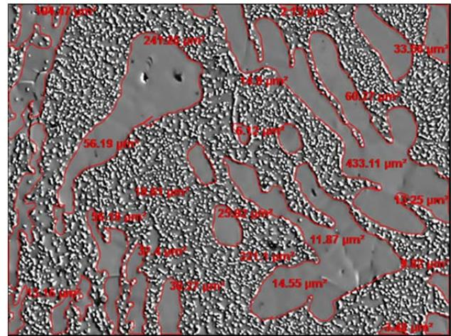
**Figure 8.** A scanning electron microscopy (SEM) image of SAC305 on Cu substrate showing how the volume fraction of the near eutectic phase can be quantified using Axiovision© or ImageJ© software.
