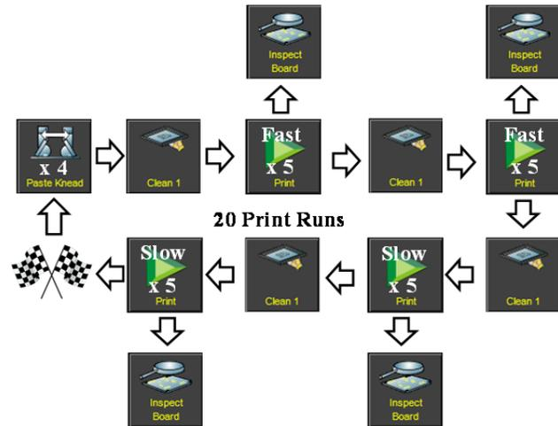
**Figure 3.** Print test sequence with 480 total prints
