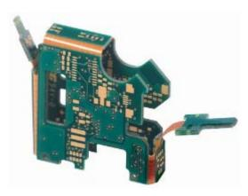
Figure 3 – Example of a Rigid-Flex PCB<sup>2</sup>
