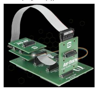
Figure 1 – 3D Assembly using Board to Board Connectors<sup>1</sup>
