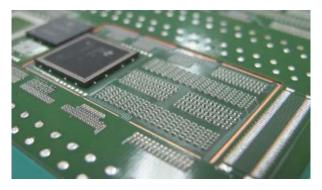
Figure 9 – Cavity Assembly
