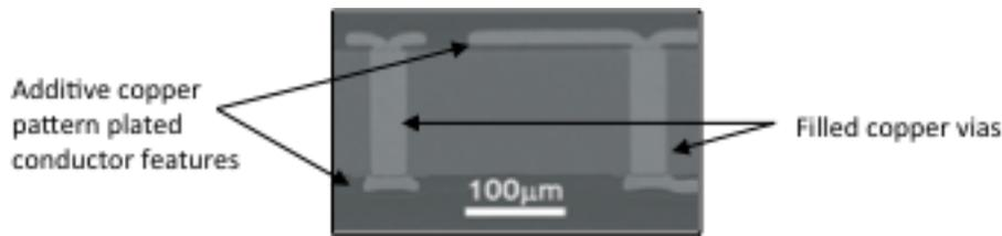
**Figure 7. Copper filled TSV interface between the interposers top and bottom surface**
