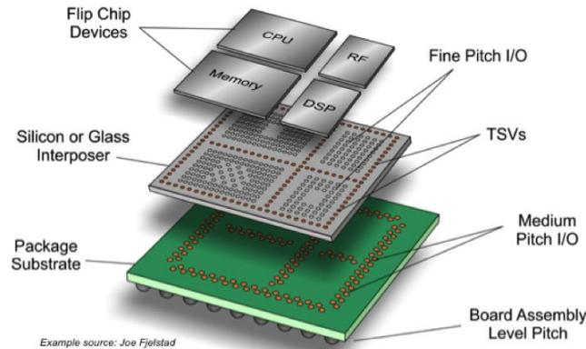
**Figure 9. General elements of a 3D system level package**
