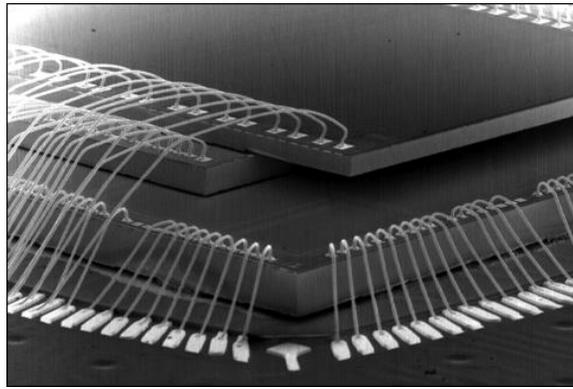
**Figure 1. Three-die, wire-bond semiconductor assembly**
