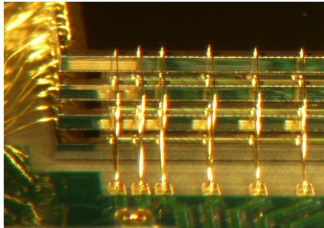
**Figure 2. Same size die stack using spacers**
