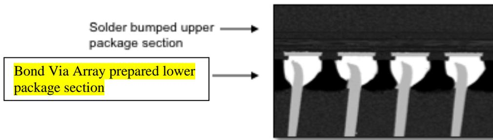
**Figure 5. Bond Via Array, Ultra Fine Pitch Copper Post Interconnect**
