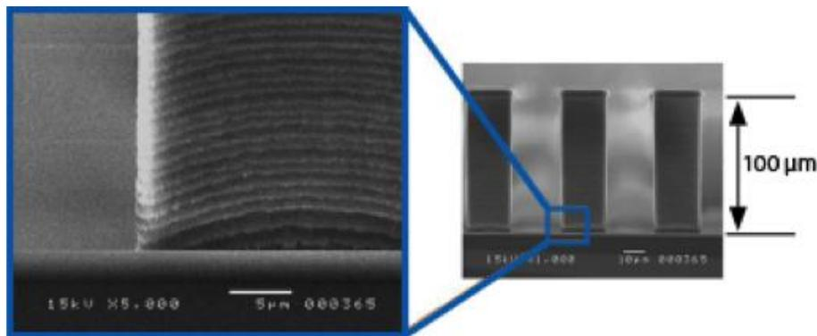
**Figure 6. Via formation using deep reactive-ion etching (DRIE) process**
