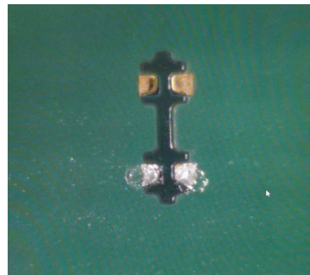
Figure 5.2 transferred solder paste to the solder pads (Source: Micro Mechanics)
