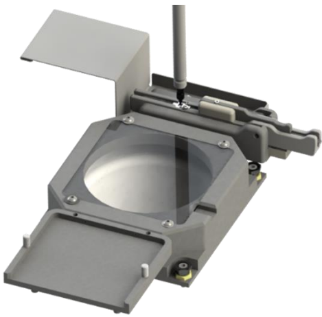
Figure 7.1 picking an 01005 from a tape feeder
