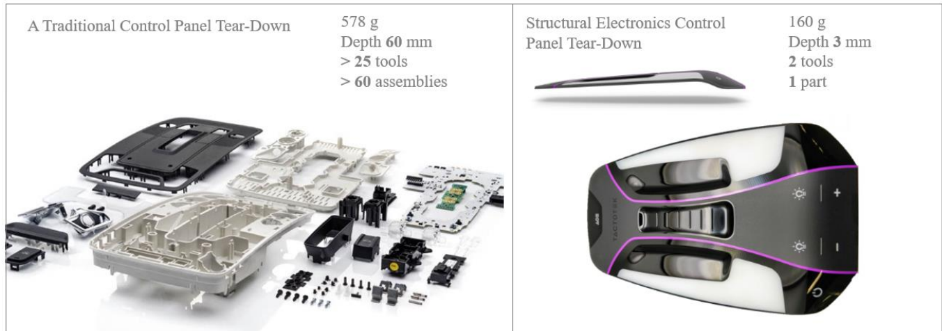
Figure 1 - Structural electronics control panel design demonstrates 70 % weight and 90 % thickness reduction when compared with conventional multi-part assembly.
