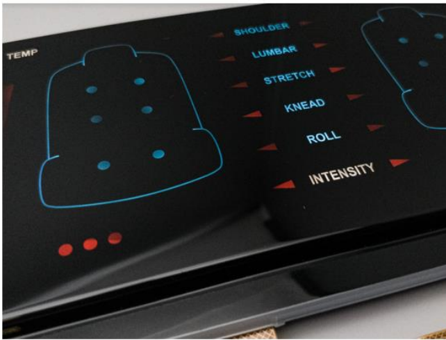
Figure 5 - Photo on left shows the back-seat-control-panel. Photo on right shows the same panel with clear A-film and injection molding resin so that electric components are visible.
