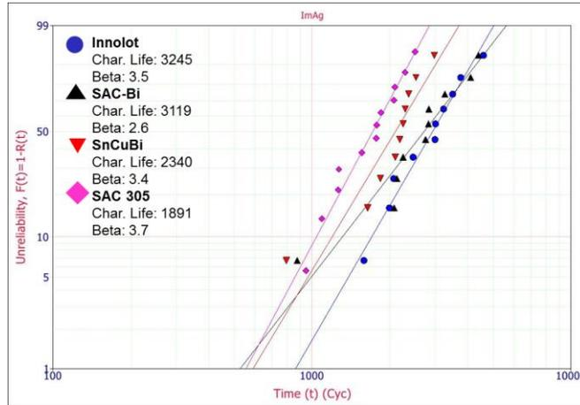
Fig. 7(a) Weibull analysis of different solder alloys with ImAg surface finish
