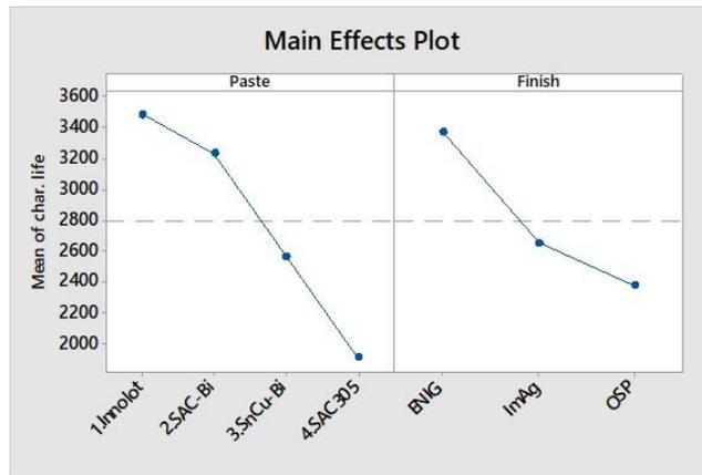
Fig. 9(a) Main effects plot for solder alloys and finishes
