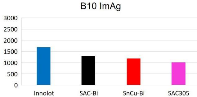
Fig. 7(c) B10 life for alloys with ImAg finish
