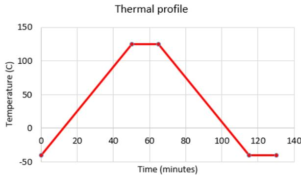
Fig. 5 Thermal cycling profile
