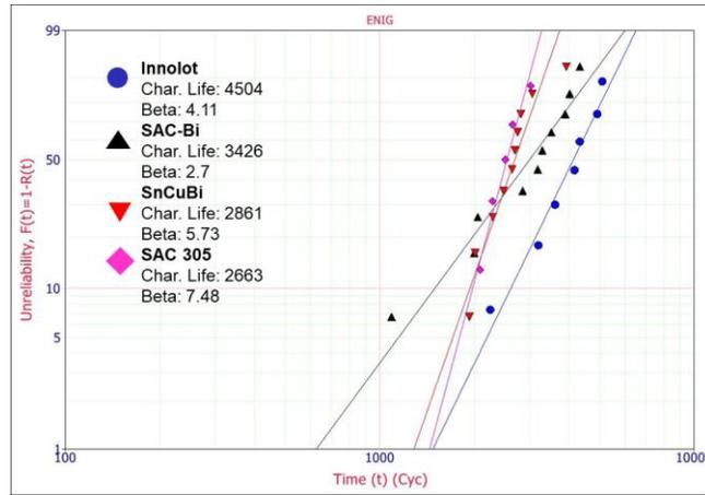
Fig. 6(a) Weibull analysis of different solder alloys with ENIG surface finish
