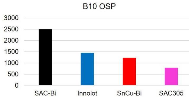
Fig. 8(c) B10 life for alloys with OSP finish
