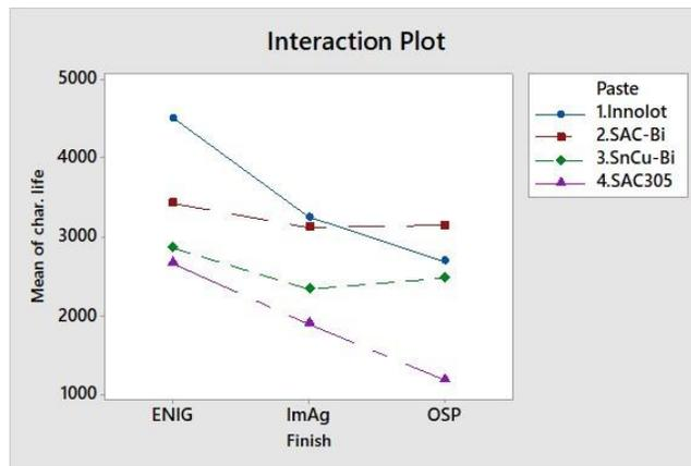
Fig. 9(b) Interaction plot for solder alloys and finishes
