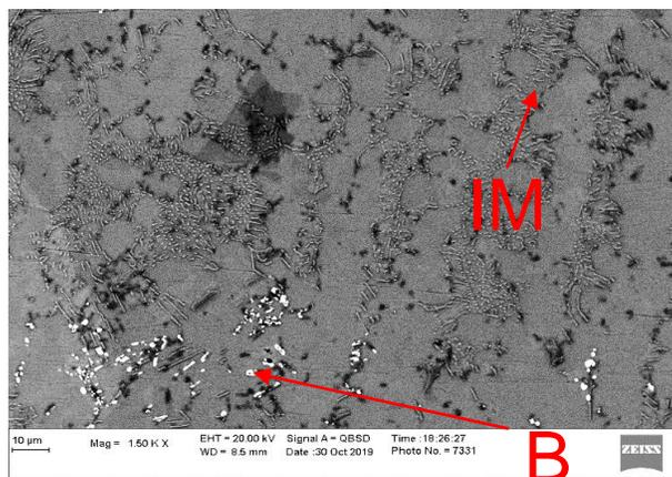
Fig. 2 Microstructure of non-aged Innolot alloy
