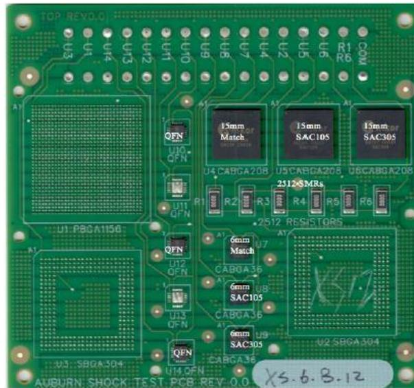
Fig. 3 Test vehicle used in the experiment
