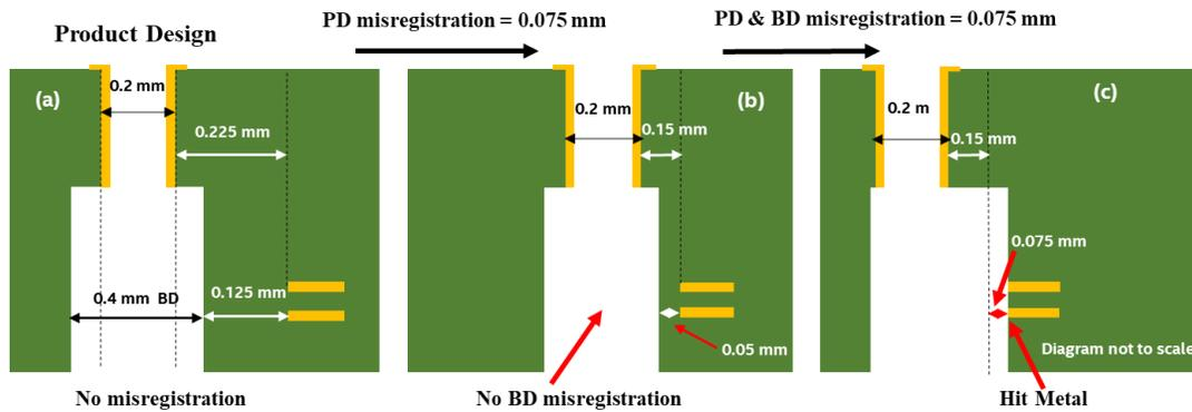
Figure 9: Example showing perfect registration, and PD and BD misregistration
