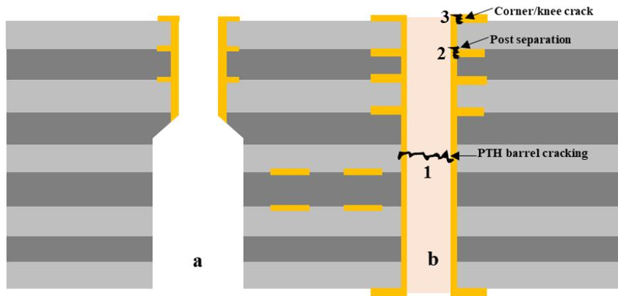
**Figure 4: Via Reliability Failure Modes**
