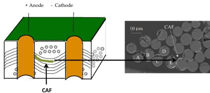
Figure 2: Traditional CAF failure for a PTH-PTH conductor orientation [4]
