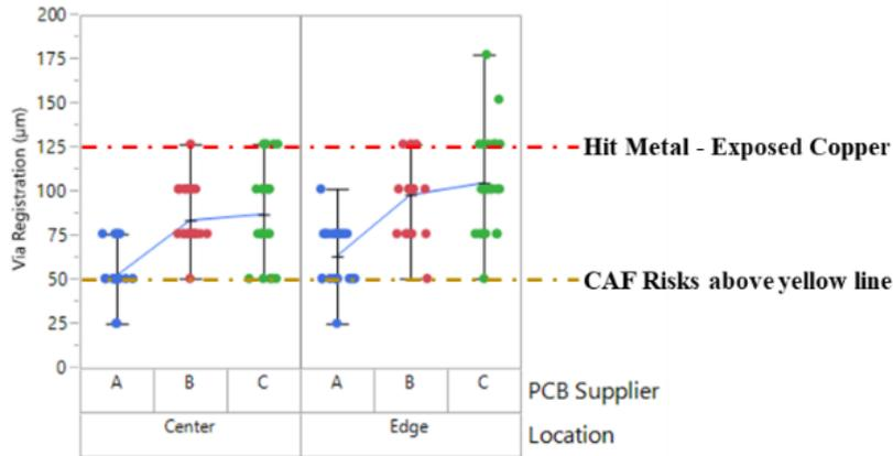
Figure 8: Variability plot showing the registration values using a PD of 200 μm for suppliers A, B, & C
