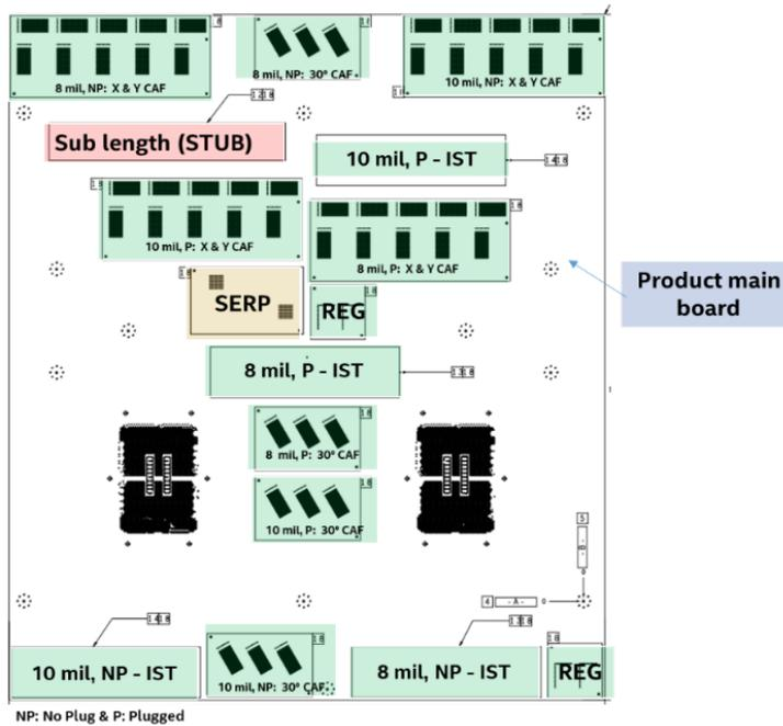
Figure 5: Layout of the DOE test vehicle with different test vehicles
