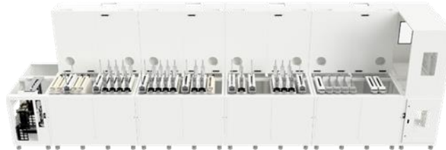
Figure 8. Panel plating tool configuration showing the series of vertical process cells
