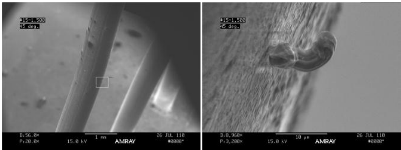
Figure 7: Typical Tin Whisker Observation (Test Specimen #15) during 500 Hour Inspection Interval
