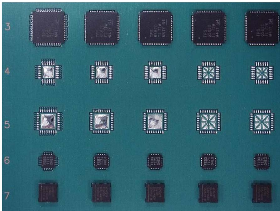
**Figure 2** Portion of the QFN Test Board
