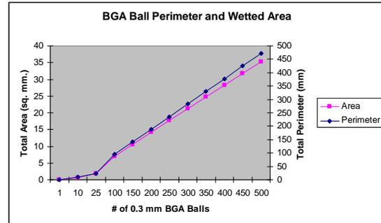
**Figure 1** Difference between Wetted Area and Wetting Perimeter as a Function of the Number of BGA Balls
