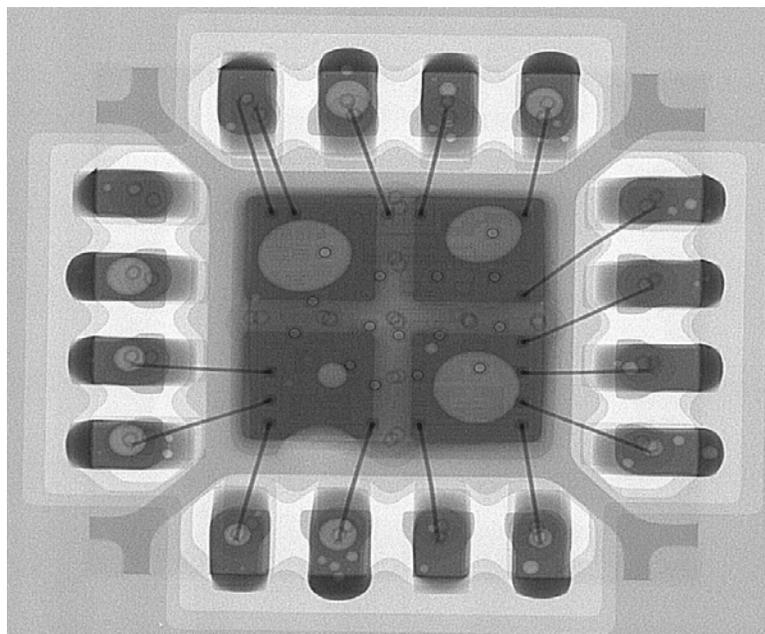
**Figure 6** X-Ray Image of PCB Test Board with QFN2 Attached
