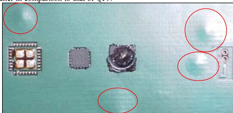
**Figure 11** Board Blistering after a total of five reflows
