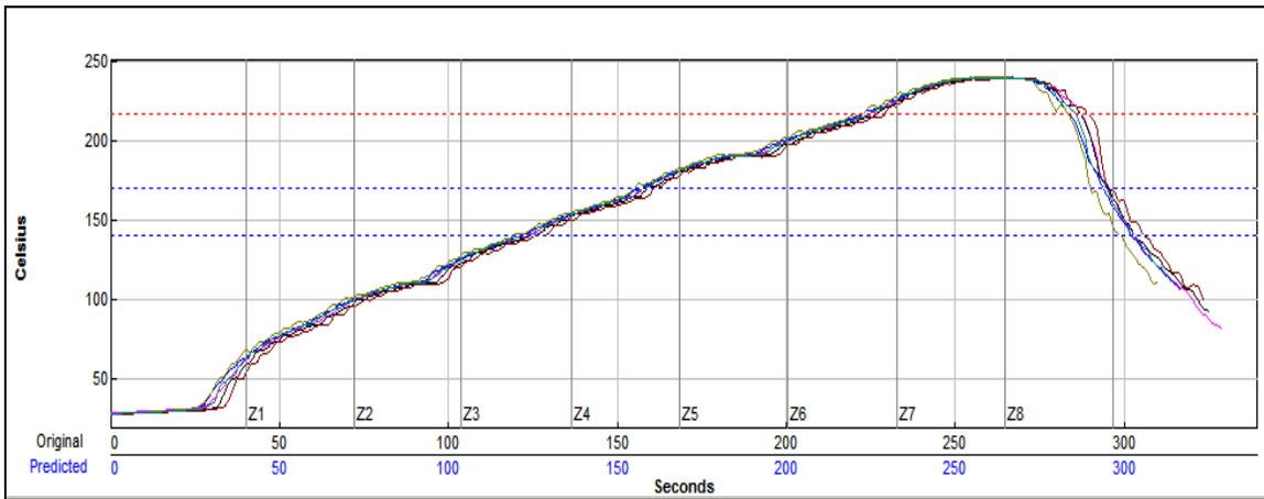
**Figure 7** Time Temperature Profile for the QFN Test Board Soldered with SAC305 developed using a Vitronics Soltec XPM3 Forced Convection Reflow Oven
