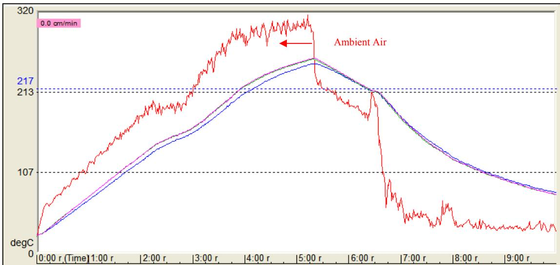
**Figure 8** Reflow Profile for the Test Board in the Pro 1600 Forced Convection Reflow Oven
