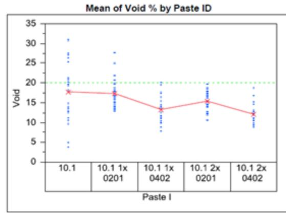
**Figure 15.** Mean values of percent voiding per condition.
