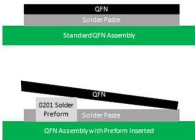
**Figure 5.** Representation of QFN component when placed with and without a solder fortification preform beneath it.
