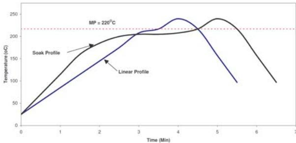
**Figure 1.** Typical soak and ramp-to-peak profiles used for lead-free solder pastes.
