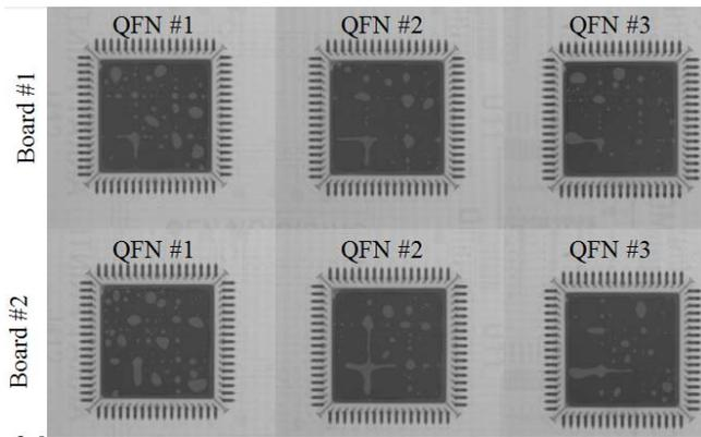
**Figure 9.** QFNs attached with solder paste, one 0402 solder fortification preform used on each.
