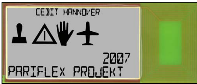
Figure 10: Display RFID demonstrator with 6 embedded chips and E ink foil (160mm X 65mm X 1mm)
