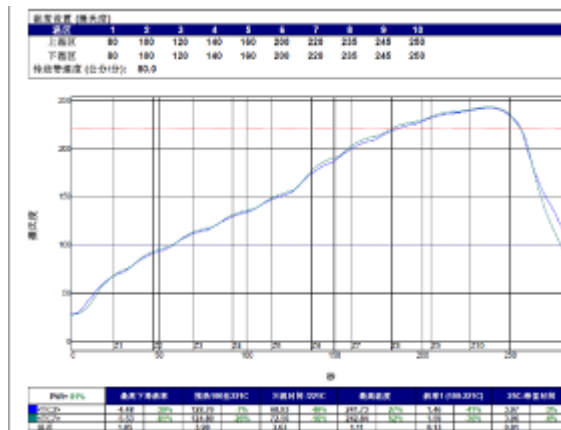
Figure 2. Reflow profile used for paste wetting test.
