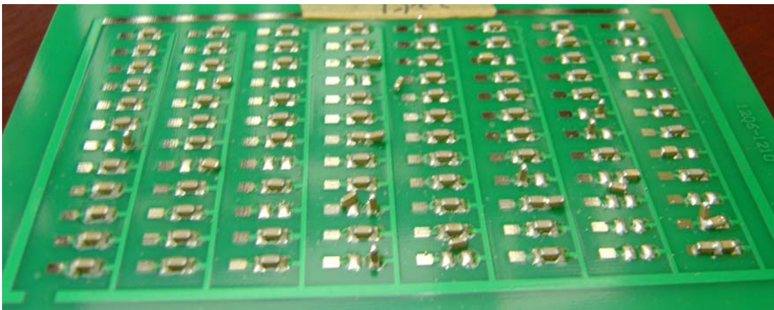
Photo 8. A test board with 96 1206 capacitors with splatter from a low cost Asia vendor
