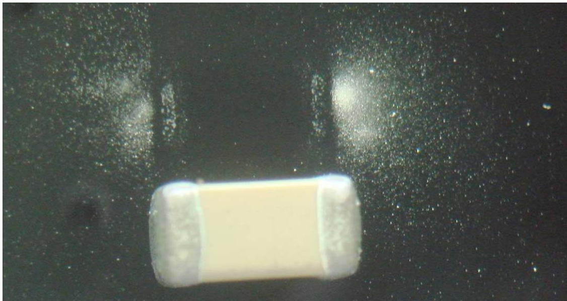
Photo 3. Another Reject from a low cost vendor part showing ejected plating salts and tin particles trapped beneath the chip
