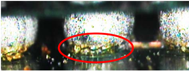
Figure 8: Crack formation – CVBGA (305) – 200TS
