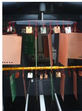
Figure 6. Chamber set up of uniformity test
