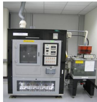
Figure 4. MFG test system in IST's lab.
