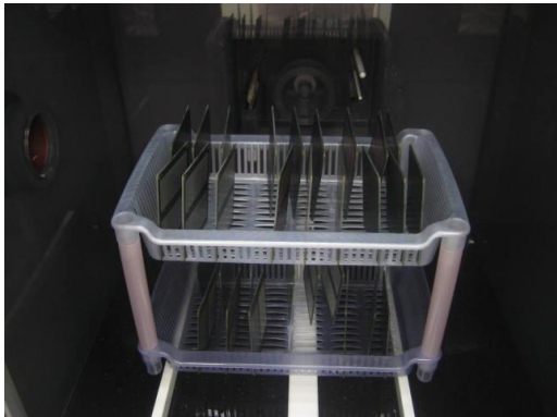
Figure 8. PCB placement for MFG Test
