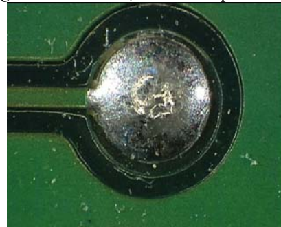
Figure 4 -No-clean, domed solder pad.
