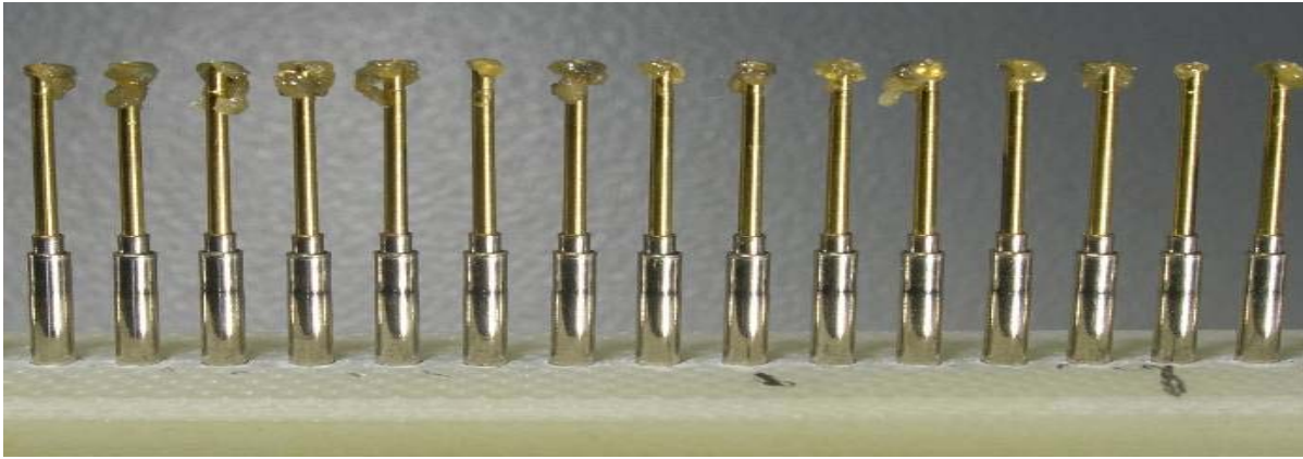
Figure 13- Razor sharp steel tip probes after 54,000 cycles still performing with a single actuation.
