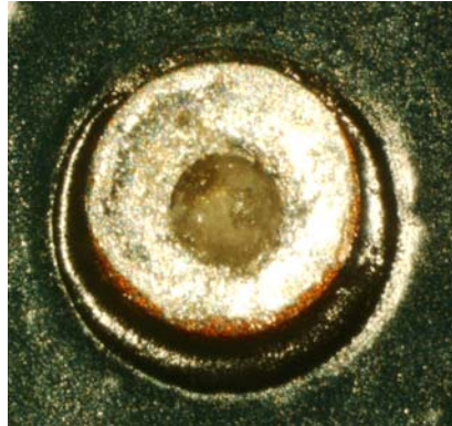
Figure 2 -Lead-free, pasted OSP via.
