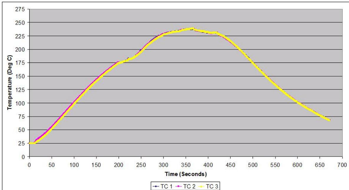
**Figure 5:** Pb Free Vapor Phase Thermal Profile used.
