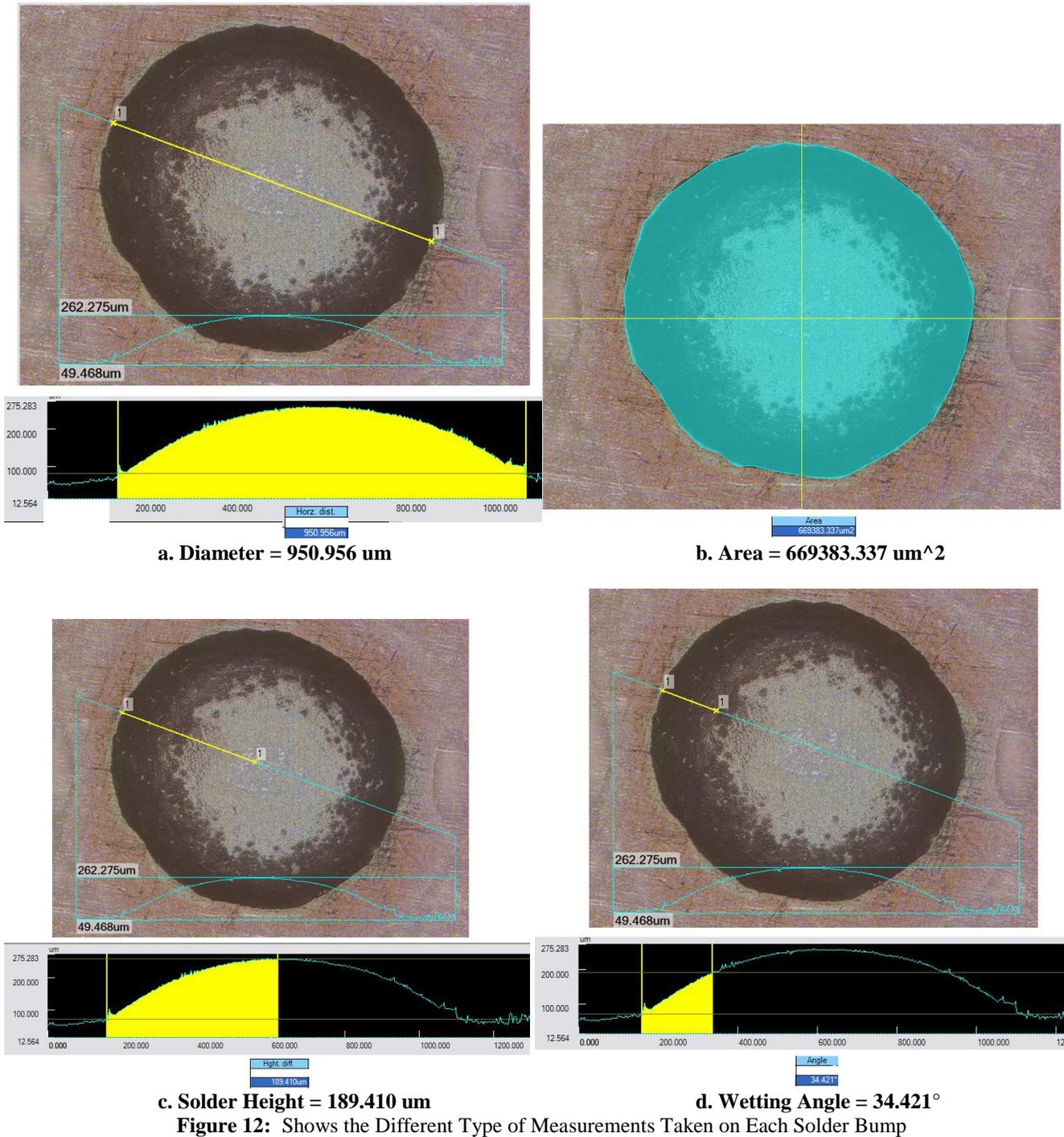
**Figure 12:** Shows the Different Type of Measurements Taken on Each Solder Bump
