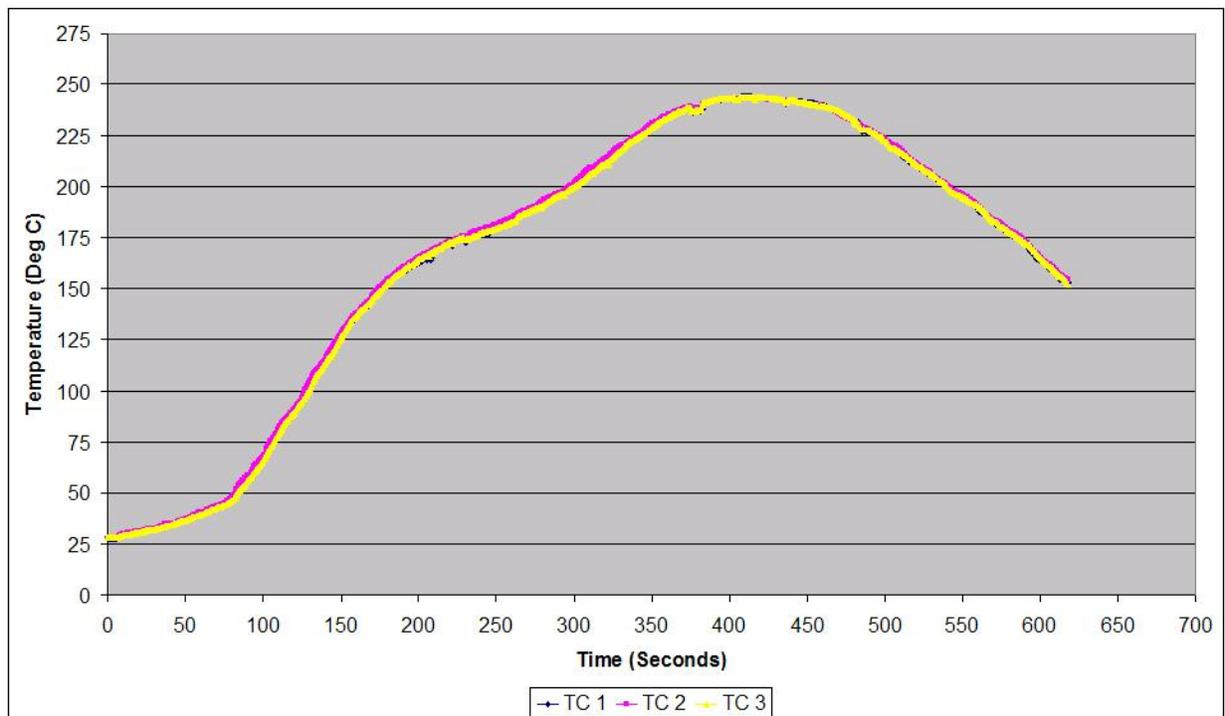
**Figure 6:** Pb Free Convection Reflow Thermal Profile used.
