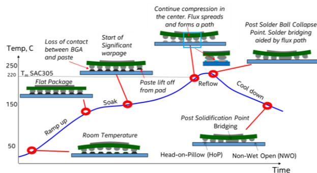
**Figure 1:** Warpage driven defect generation mechanism
