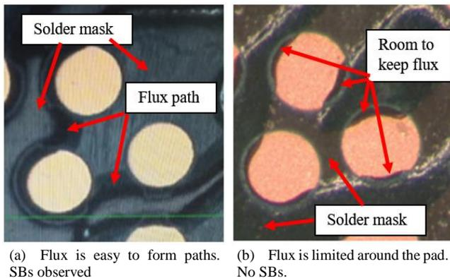
**Figure 3.** Pad design impacts availability of flux between solder pads to provide a path for solder to bridge
