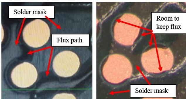
**Figure 3.** Pad design impacts availability of flux between solder pads to provide a path for solder to bridge
