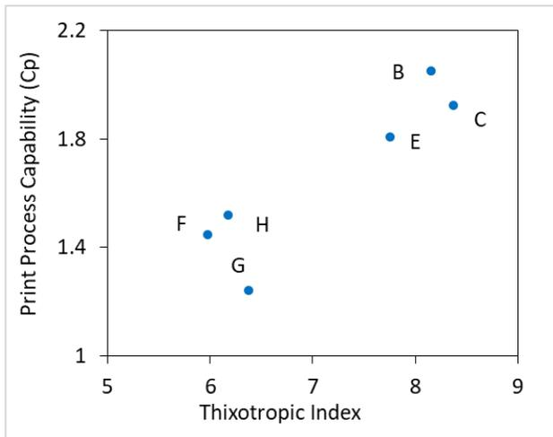
**Figure 12:** Plot of the Thixotropic Index vs the Print Process Capability ( $C_p$ ). For all 8 solder pastes evaluated.
