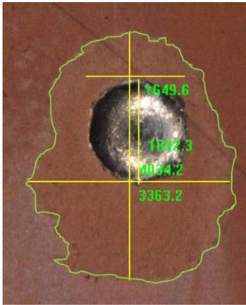
**Figure 6:** Representative image of the CuOSP solder spread test showing solder spread and flux spread (green outline) measurements using maximum spread diameters perpendicular to each other
