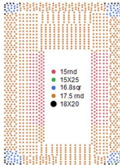
**Figure 2.** Multiple Aperture Sizes for a BGA (center is 15 mil circle, while corner is up to 18X20 rectangular)
