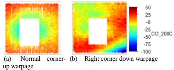
**Figure 4.** Two different packages from same lot with significantly different warpage profile at high temperature (200°C). The scale bar shows warpage numbers in um.
