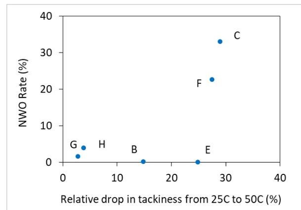
**Figure 8:** Drop in tackiness showed a mild correlation with NWO rate with the 2 worst performing pastes showing the largest relative drops in tack force from room temperature to high temperature.
