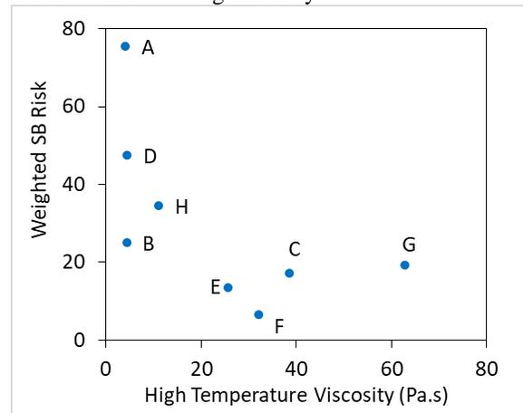
**Figure 11:** Plot of the High Temperature Viscosity vs the Weighted Solder Bridging Risk for all 8 solder pastes evaluated.
