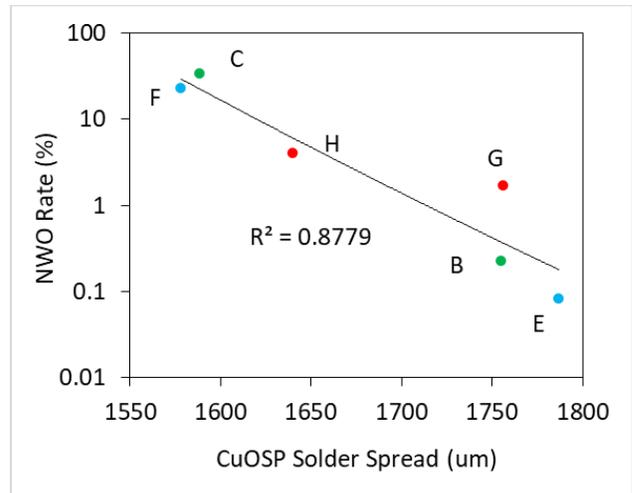
**Figure 7:** Plot of the Pin level NWO rate (on a log scale) and CuOSP solder spread. A logarithmic correlation is observed. Red, blue and green colors represent halogenated, halogen free compliant and zero halogen pastes respectively.
