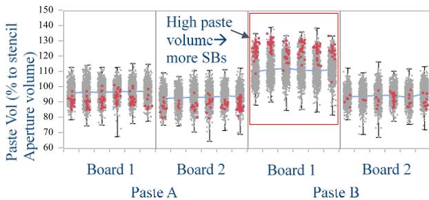
**Figure 10.** The variability chart of Paste Volume% for two different pastes on two different boards. Red dots represent paste volume for pins with bridging defects. Others are no bridging pins.
