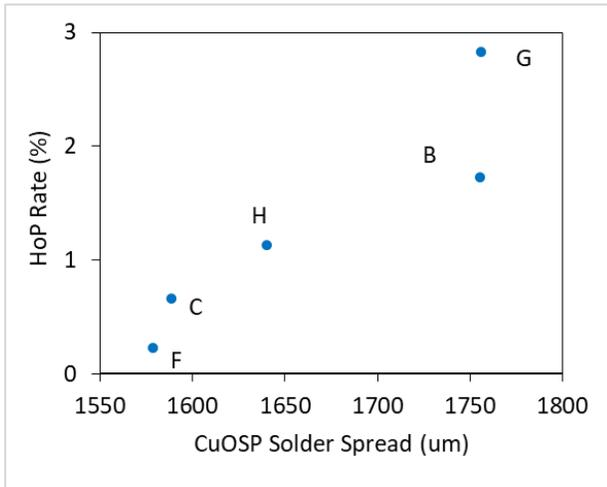
**Figure 9:** Pin level HoP defect rate showed inverse correlation with the CuOSP solder spread
