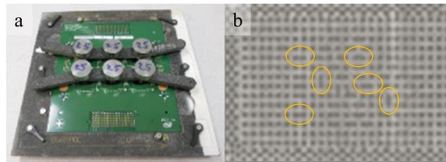
**Figure 5:** (a) Hammer test setup fixture with weights to compress in the middle of the package to force solder bridging during SMT reflow (b) A few of the bridging defects have been highlighted in a typical X-ray image in the center of the package post SMT.
