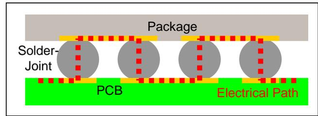
**Figure 1.** A daisy-chain connection representation between package substrate bottom metal and printed circuit board top metal. The red dashed line illustrates the electrical path.
