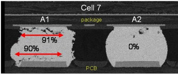
**Figure 11.** Cross-section of corner solder-joint A1 and neighbor A2 from 292MAPBGA cell 7 (large 11mil die with SAC387 ball) after 3000 cycles. The corner solder-joint was distorted and had significant cracking at both the package and PCB sides, but the neighbor had no appreciable damage.
