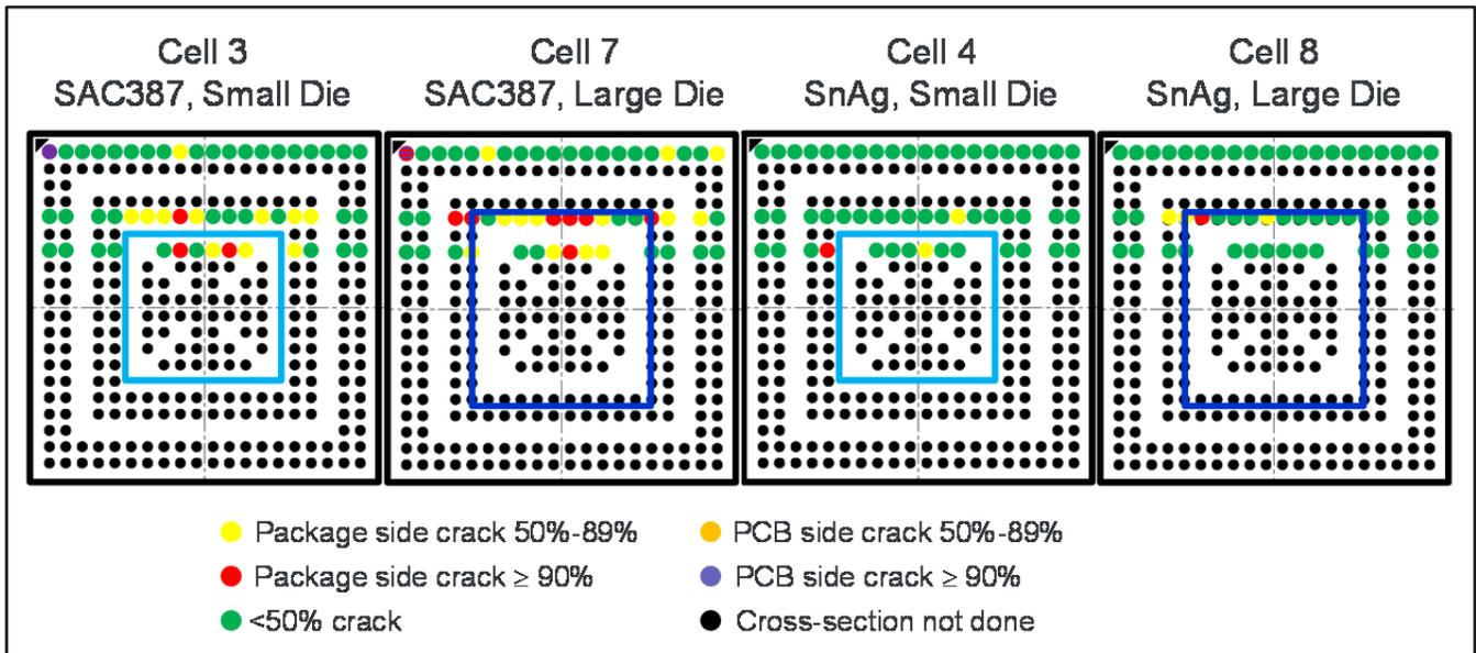
Figure 12. Degree of cracking distribution from cross-section for 292MAPBGA 11mil thick die cells after 3000 cycles.
