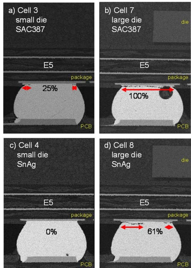
**Figure 9.** Cross-section of 292MAPBGA solder-joint E5 after 3000 cycles. All with 11mil thick die. Solder-joints in proximity to the die edge (cells 7 and 8) had larger cracks.
