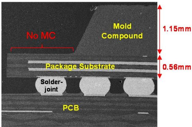
**Figure 3.** Typical 512TEPBGA cross-section.
