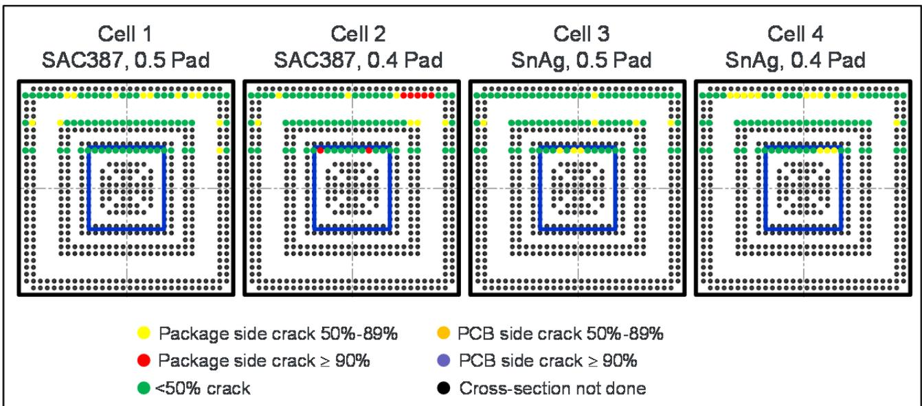
Figure 19. Degree of cracking distribution from cross-section for 512TEPBGA 11mil thick die cells after 3164 cycles.
