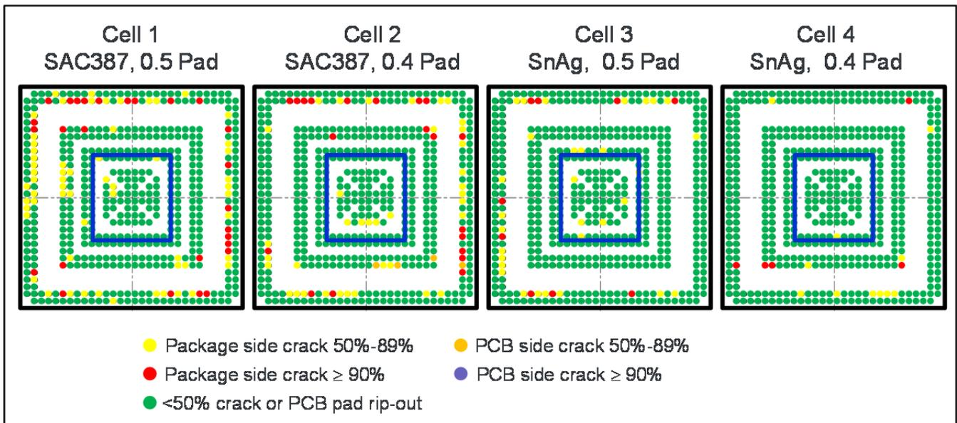
Figure 20. Degree of cracking distribution from dye-and-pry for 512TEPBGA 11mil thick die cells after 4073 cycles.
