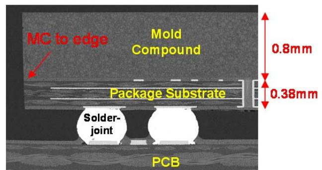
**Figure 2.** Typical 292MAPBGA cross-section.
