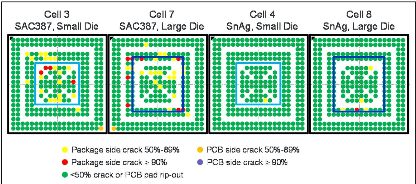
Figure 13. Degree of cracking distribution from dye-and-pry for 292MAPBGA 11mil thick die cells after 4000 cycles.
