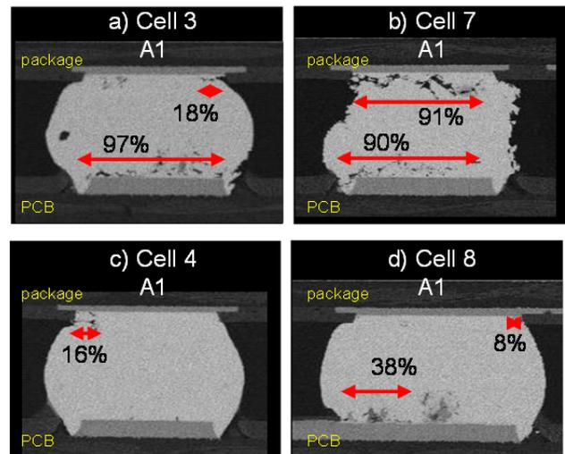
**Figure 10.** Cross-section of typical 292MAPBGA corner solder-joints after 3000 cycles. a) small die SAC387, b) large die SAC387, c) small die SnAg, d) large die SnAg. All with 11mil thick die. Note the propensity for cracking on the PCB side and the distorted solder-joint shapes.
