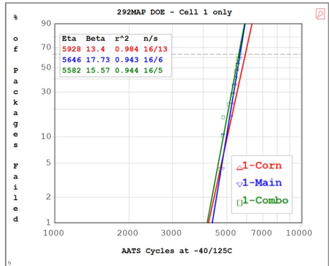
**Figure 7.** 292MAPBGA cell 1. The corner net, main net and combined distributions are nearly identical.
