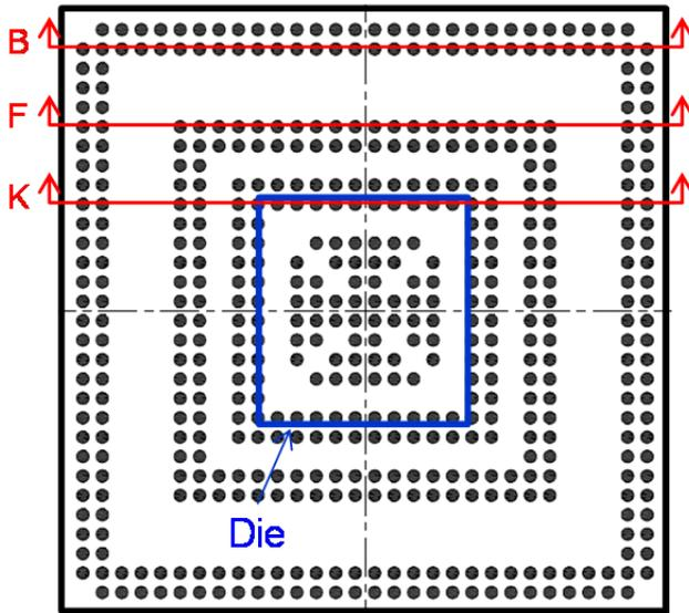
Figure 16. 512TEPBGA Cross-section locations.
