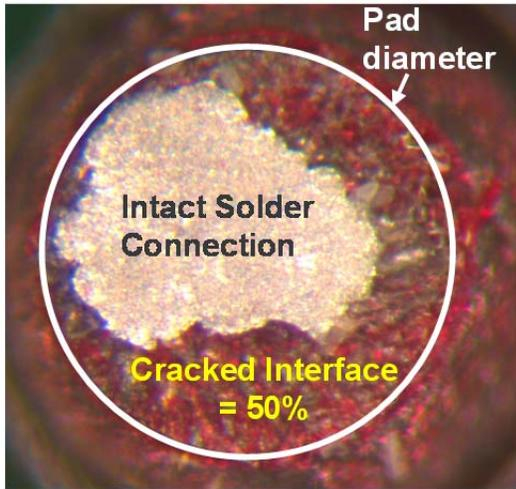
**Figure 5.** Example dye-and-pry image and degree of cracking calculation.
