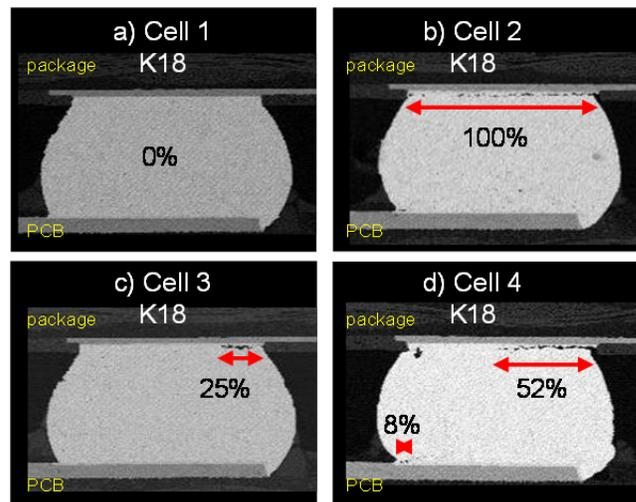
Figure 18. Cross-section of typical 512TEPBGA row K (under die edge) solder-joints after 3164 cycles. a) SAC387 0.5mm, PCB pad, b) SAC387 0.4mm, PCB pad, c) SnAg, 0.5mm, PCB pad, d) SnAg, 0.4mm, PCB pad,. All with 11mil thick die.
