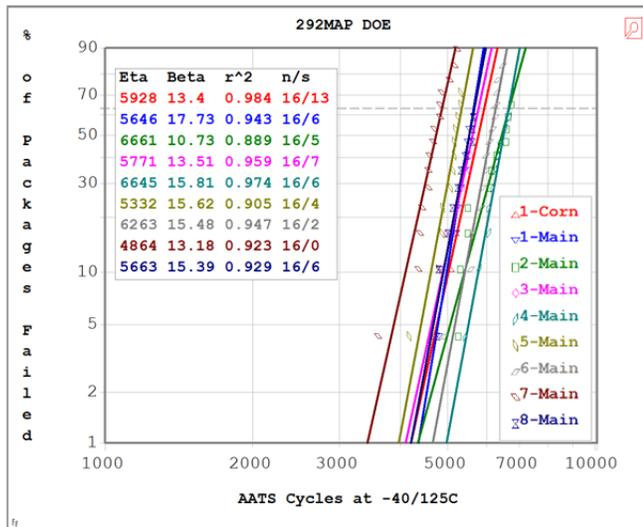
**Figure 6.** 292MAPBGA Weibull plots for all cells and nets. Only cell 1 had more than one corner net failures.
