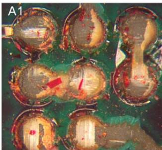
**Figure 14.** Example corner dye-and-pry on 292MAPBGA after 4000 cycles. This image is viewing the PCB surface.
