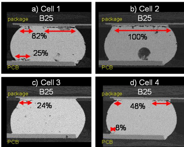
Figure 17. Cross-section of typical 512TEPBGA row B solder-joints after 3164 cycles. a) SAC387 0.5mm, PCB pad, b) SAC387 0.4mm, PCB pad, c) SnAg, 0.5mm, PCB pad, d) SnAg, 0.4mm, PCB pad,. All with 11mil thick die.
