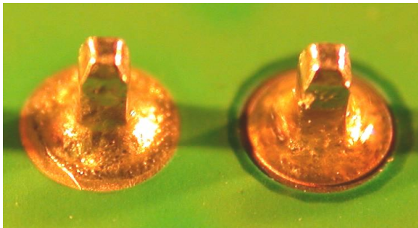
Figure 7. The solder preform + solder paste solution delivered excellent through-hole solder joints.
