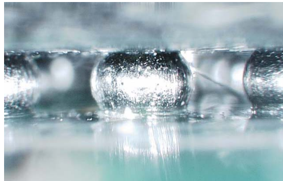
Figure 3: Magnified view of a reflowed BGA
