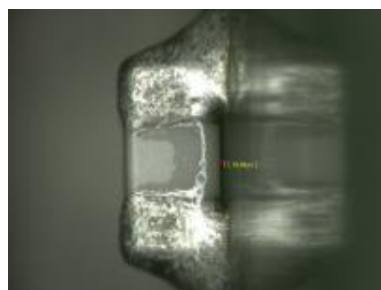
Figure 3. 0402 component standoff: 20 microns or 0.8 mil
