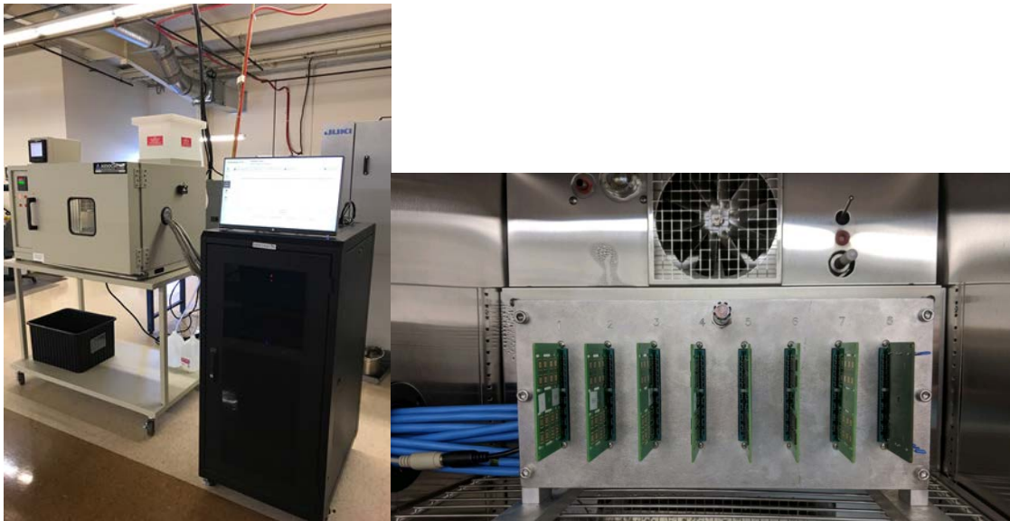
Figure 8: Test Instrument (Left) and Fixture (Right) Located in the Environmental Chamber
