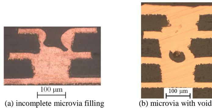
**Figure 2 - Examples of Microvia Filling Issues**
