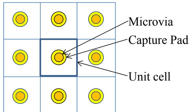
**Figure 3 - Illustration of a Unit Cell**
