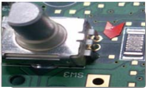
Figure 22. Insufficient hole penetration
