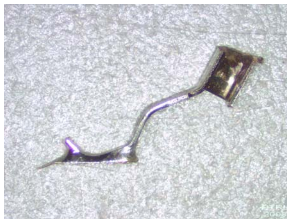
Figure 7 Typical pin with copper pad attached
